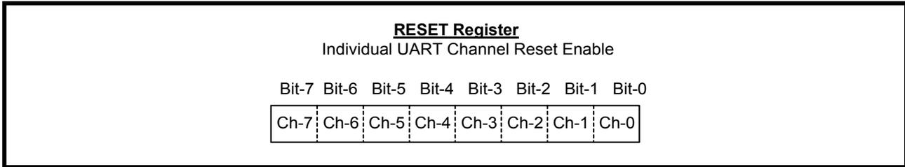
The 8-bit RESET register provides the software with the ability to reset the UART(s) when there is a need. Each bit is self-resetting after it is written a logic 1 to perform a reset to that channel. All registers in that channel will be reset to the default condition, see **Table 19** for details. As an example, bit-0 =1 resets UART channel 0 with bit-7=1 resets channel 7.
