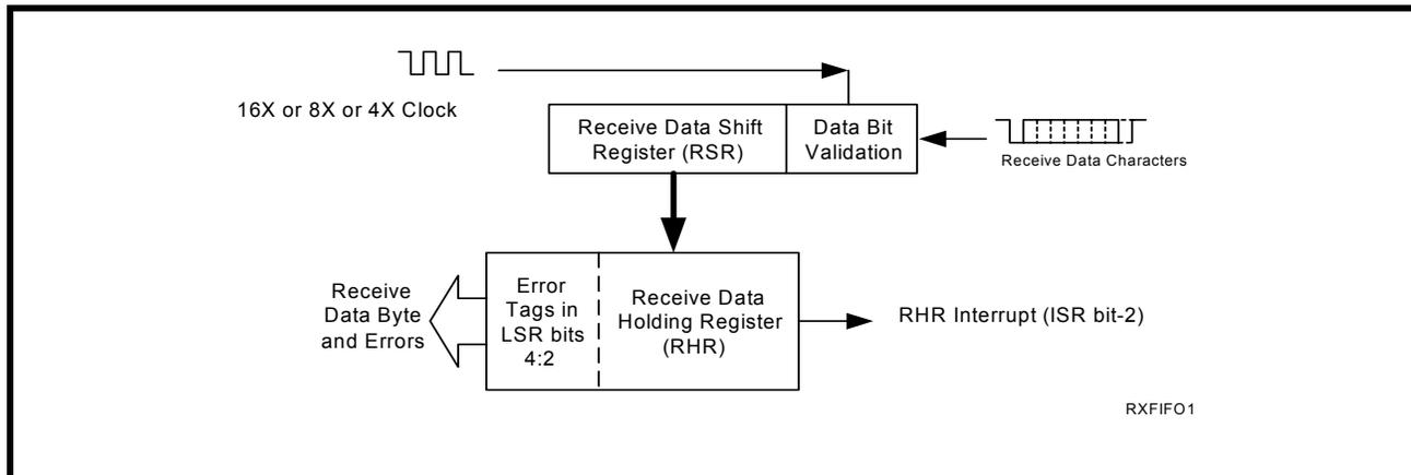
**FIGURE 8. RECEIVER OPERATION IN FIFO AND AUTO RTS FLOW CONTROL MODE**
