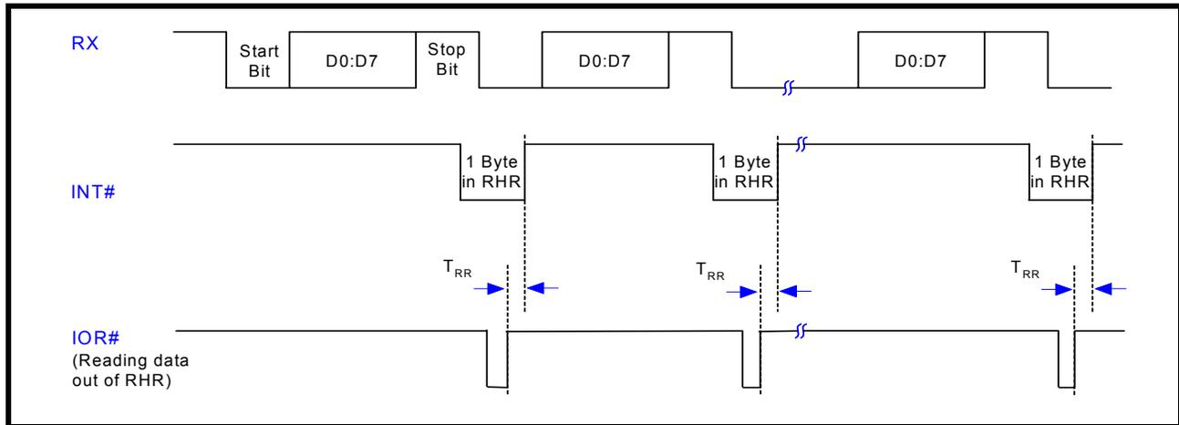
FIGURE 20. TRANSMIT INTERRUPT TIMING [NON-FIFO MODE]
