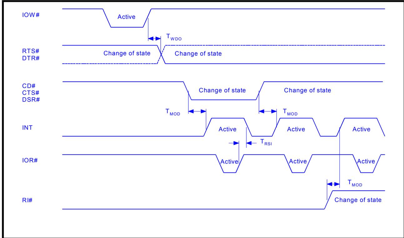
FIGURE 19. RECEIVE INTERRUPT TIMING [NON-FIFO MODE]
