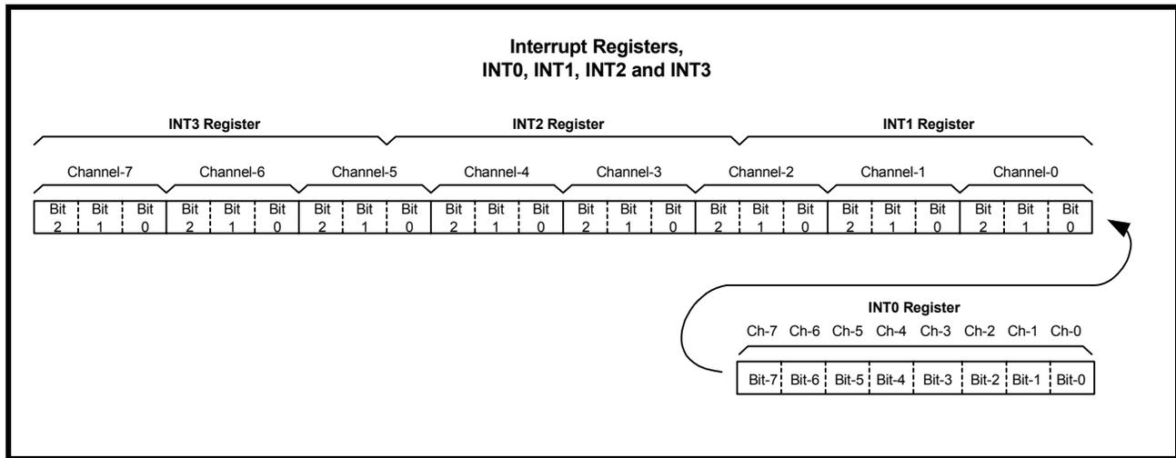
**TABLE 10: UART CHANNEL [7:0] INTERRUPT SOURCE ENCODING AND CLEARING**
