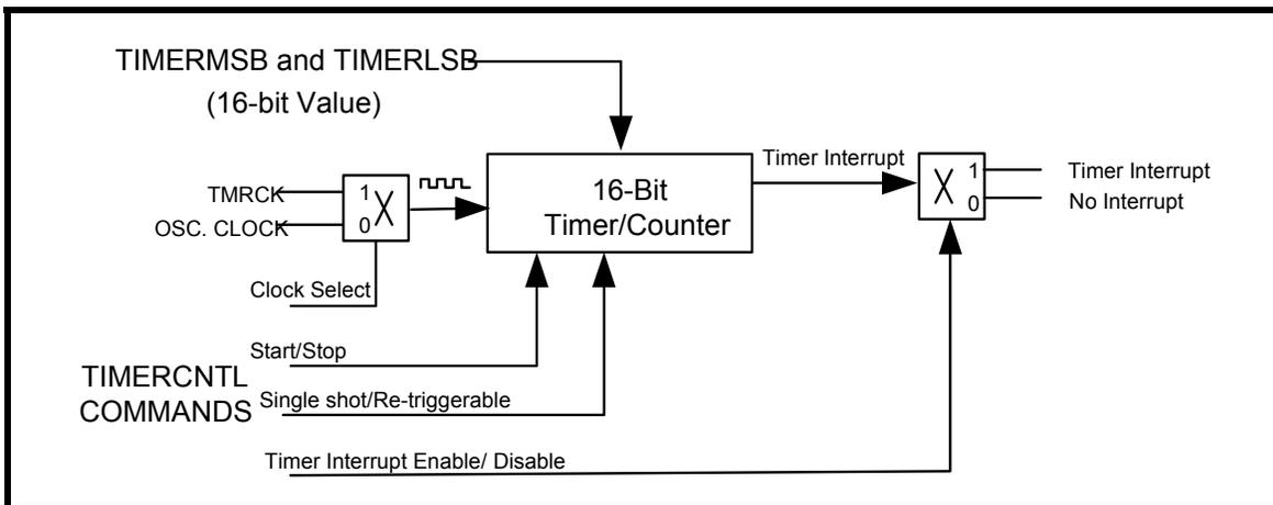
FIGURE 15. INTERRUPT OUTPUT IN ONE-SHOT AND RE-TRIGGERABLE MODES
