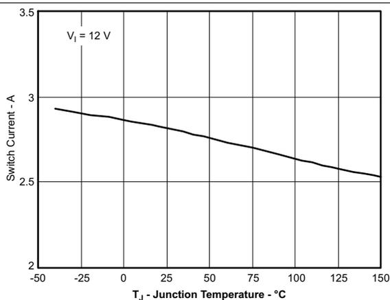
Figure 3. Switch Current Limit vs Junction Temperature
