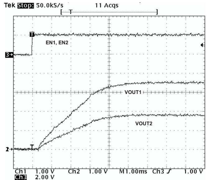
Figure 33. Ratio-Metric Startup using Coupled SS/TR pins
