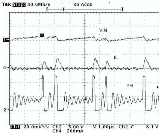
Figure 59. Input Ripple PSM
