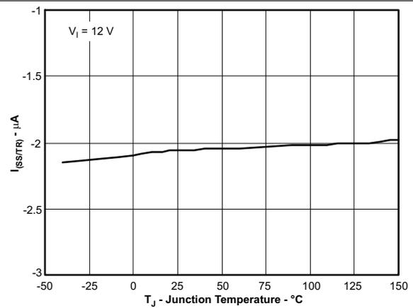
Figure 12. SS/TR Charge Current vs Junction Temperature
