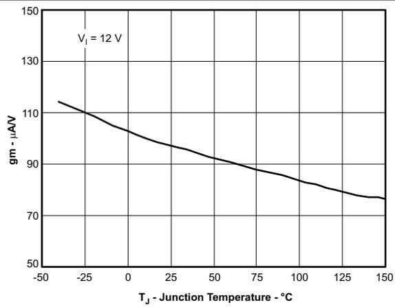
Figure 8. EA Transconductance vs Junction Temperature
