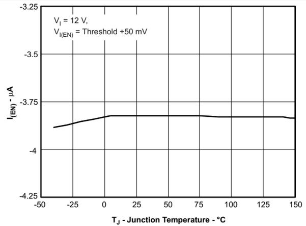
Figure 10. EN Pin Current vs Junction Temperature
