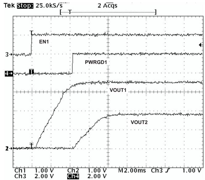
Figure 31. Sequential Startup using EN and PWRGD
