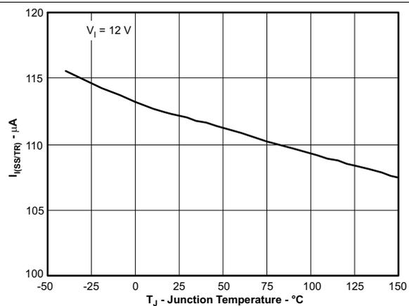
Figure 13. SS/TR Discharge Current vs Junction Temperature
