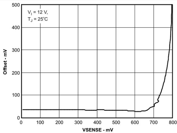
Figure 23. SS/TR to VSENSE Offset vs VSENSE
