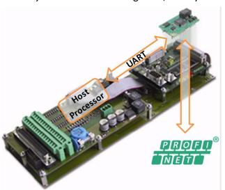
Software integration with a Host processor is also easy since no re-programming is required on the Host processor and the Host firmware is never touched. The *RapID Universal Gateway* conforms to the Host messages passed over the UART by using a "script". This script transforms the UART messages into the appropriate Profinet messages. Simply write a script to interpret the UART messages and the field device is ready to talk on the network.
