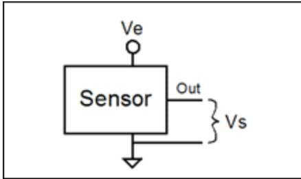
Figure 1. Generic ratiometric sensor.
