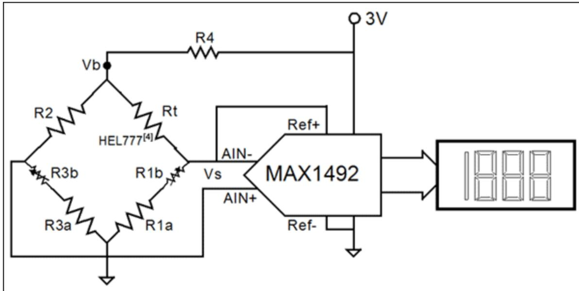
Figure 10. In this simple temperature sensor with a digital display, the bridge circuit removes the unwanted signal at 0°, which allows the ADC reading to equal the temperature.
