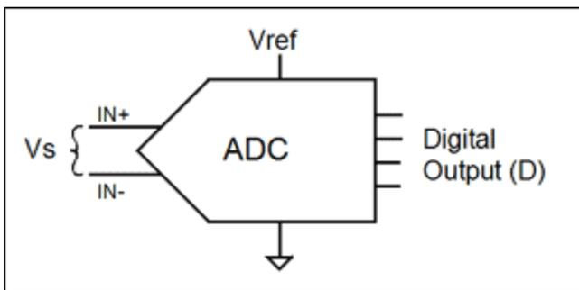
Figure 2. Generic analog-to-digital converter.
