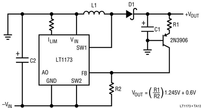
Figure 8. Negative-to-Positive Converter
