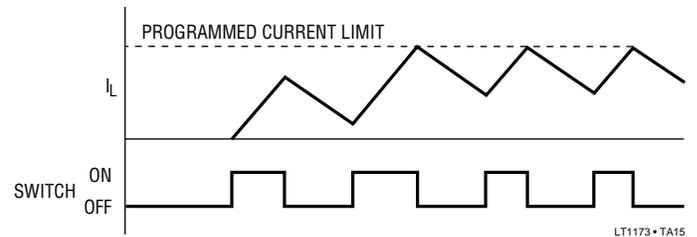
Figure 10. Current Limit Keeps Inductor Current Under Control
