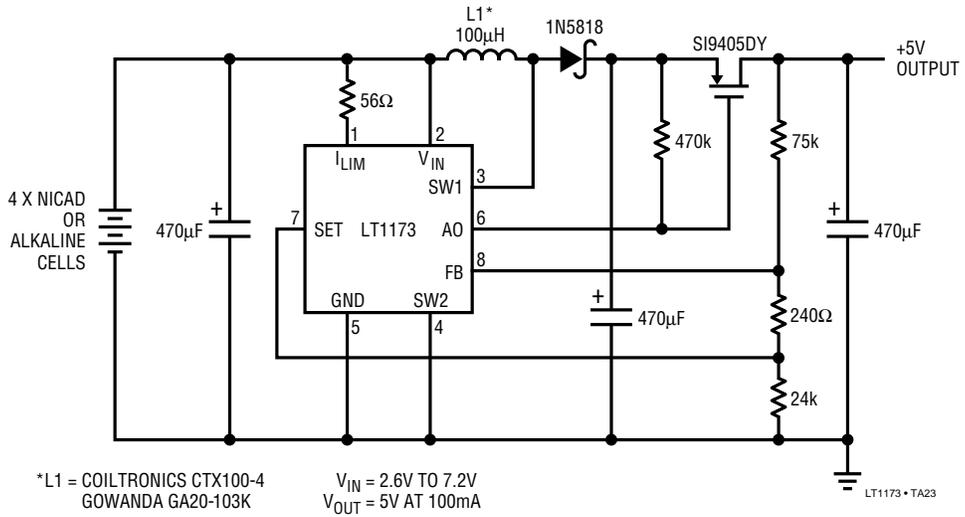
2V to 5V at 300mA Step-Up Converter with Under Voltage Lockout
