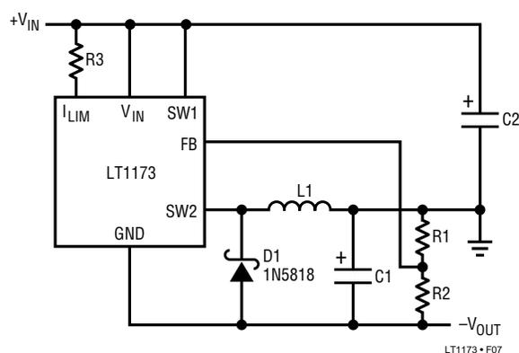
Figure 7. Positive-to-Negative Converter
