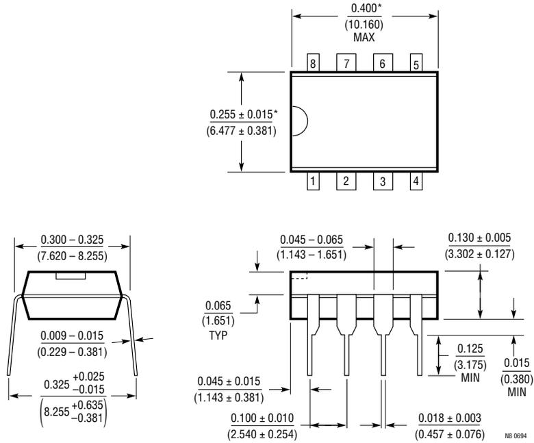
\*THESE DIMENSIONS DO NOT INCLUDE MOLD FLASH OR PROTRUSIONS.
