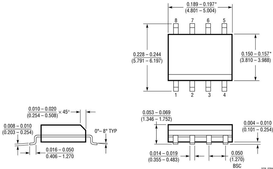
\*THESE DIMENSIONS DO NOT INCLUDE MOLD FLASH OR PROTRUSIONS.
