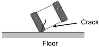
3. When printed circuit boards are piled up or handled, the corners of another printed circuit board should not be allowed to hit the capacitor in order to avoid a crack or other damage to the capacitor.
