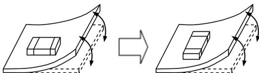
Locate chip horizontal to the direction in which stress acts
