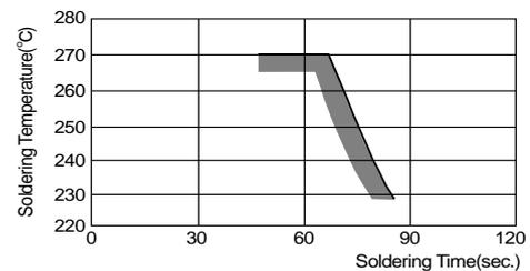
In case of repeated soldering, the accumulated soldering time must be within the range shown above.
