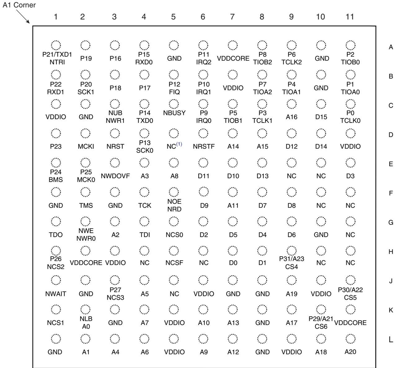
Note: 1. Not connected, can either be connected to GND, VCC or left unconnected.
