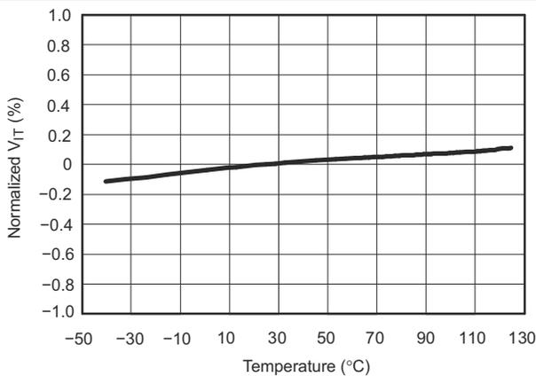
**Figure 7-6. Normalized Sense Threshold Voltage ( $V_{IT}$ ) vs Temperature**
