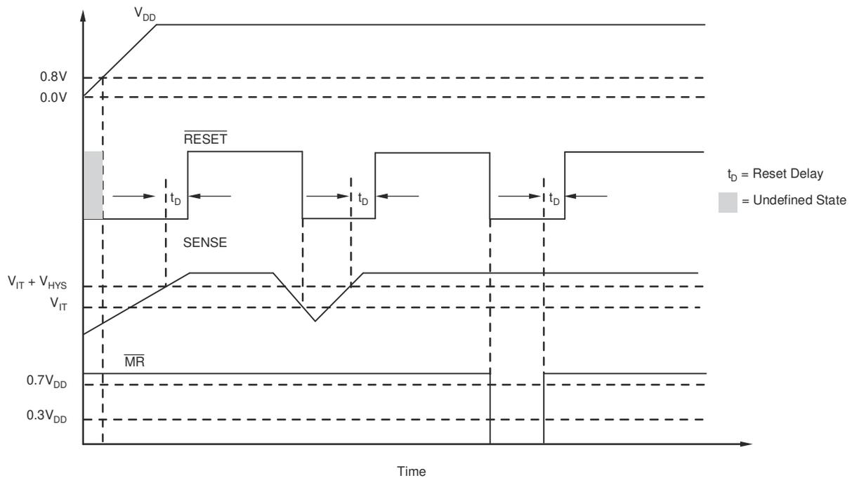
**Figure 7-1. TPS3808 Timing Diagram Showing  $\overline{\text{MR}}$  and SENSE Reset Timing**
