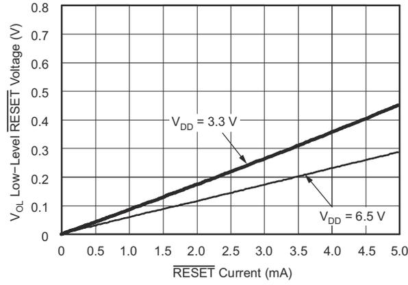
**Figure 7-8. Low-Level  $\overline{RESET}$  Voltage vs  $\overline{RESET}$  Current**
