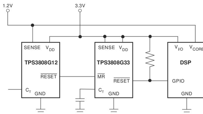
Figure 8-3. Using  $\overline{MR}$  to Monitor Multiple System Voltages
