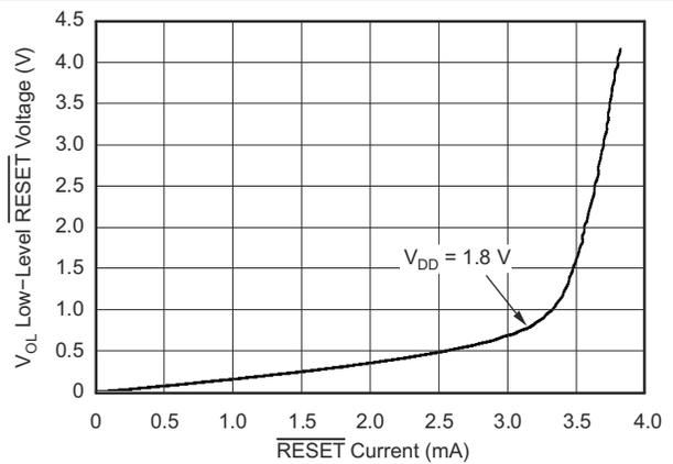
**Figure 7-7. Low-Level RESE Voltage vs RESE Current**
