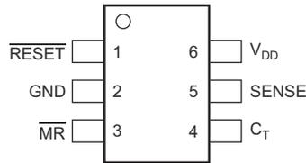
Figure 6-1. DBV Package 6-Pin SOT-23 Top View
