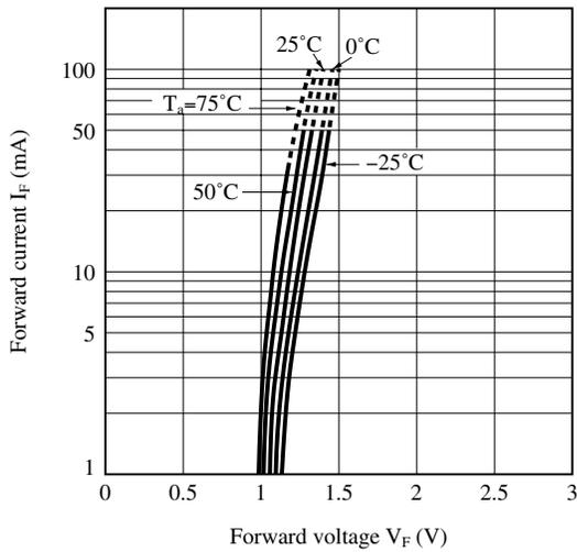
**Fig.3-b Forward Current vs. Forward Voltage (Rank 2)**
