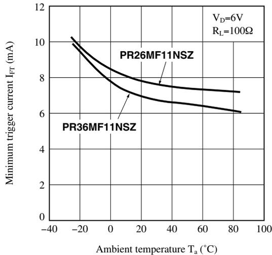
**Fig.4-b Minimum Trigger Current vs. Ambient Temperature (Rank 2)**
