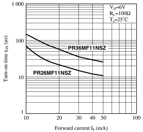
**Fig.8-b Turn-on Time vs. Forward Current (Rank 2)**
