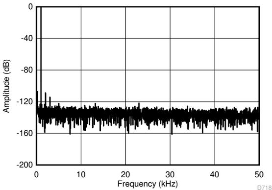
$f_{\text{SAMPLE}} = 100 \text{ kSPS}$ ,  $V_{\text{IN}} = \pm 12 \text{ V}$ ,  $f_{\text{IN}} = 1 \text{ kHz}$ ,  $V_{\text{CM}} = 50 \text{ V}_{\text{DC}}$ ,
