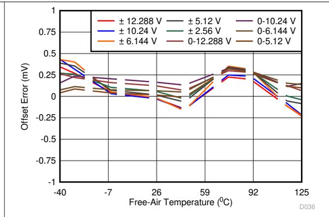
Figure 6-28. Offset Error vs Temperature Across Input Ranges
