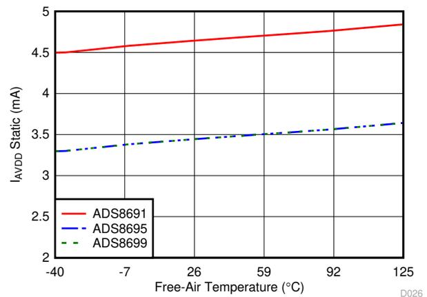
Figure 6-44. AVDD Current vs Temperature (During Sampling)
