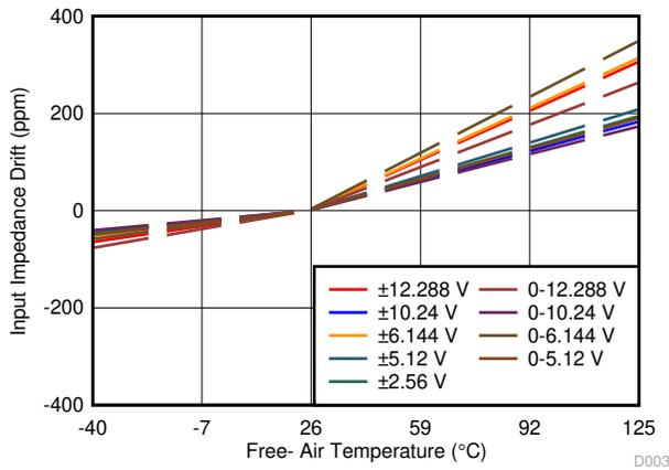
Figure 6-11. Input Impedance Drift vs Temperature
