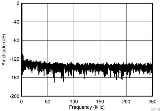
$f_{\text{SAMPLE}} = 500 \text{ kSPS}$ ,  $V_{\text{IN}} = \pm 12 \text{ V}$ ,  $f_{\text{IN}} = 1 \text{ kHz}$ ,  $V_{\text{CM}} = 50 \text{ V}_{\text{DC}}$ ,
