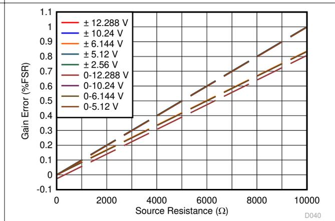
Figure 6-32. Gain Error vs External Resistance ( $R_{EXT}$ )
