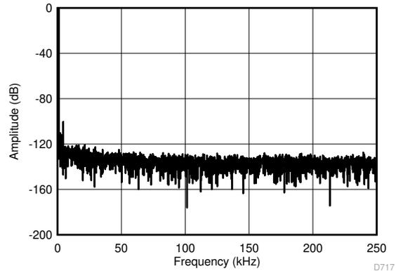
$f_{\text{SAMPLE}} = 500 \text{ kSPS}$ ,  $V_{\text{IN}} = \pm 12 \text{ V}$ ,  $f_{\text{IN}} = 1 \text{ kHz}$ ,  $V_{\text{CM}} = 155 \text{ V}_{\text{PP}}$ ,
