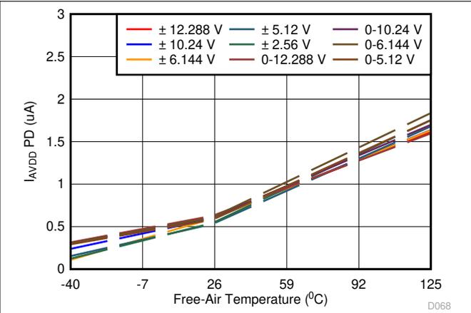
Figure 6-46. AVDD Current vs Temperature (Power-Down Mode)
