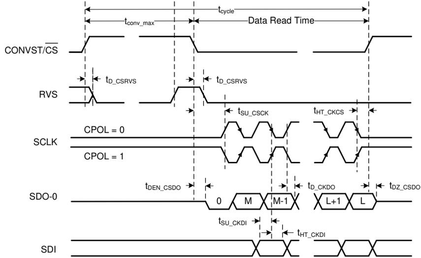
**Figure 6-4. Standard SPI Interface Timing Diagram for CPHA = 1**
