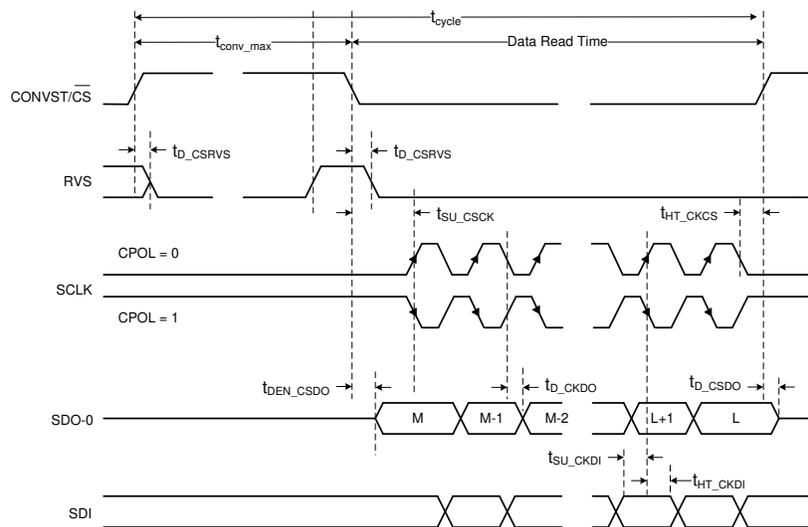
**Figure 6-3. Standard SPI Interface Timing Diagram for CPHA = 0**
