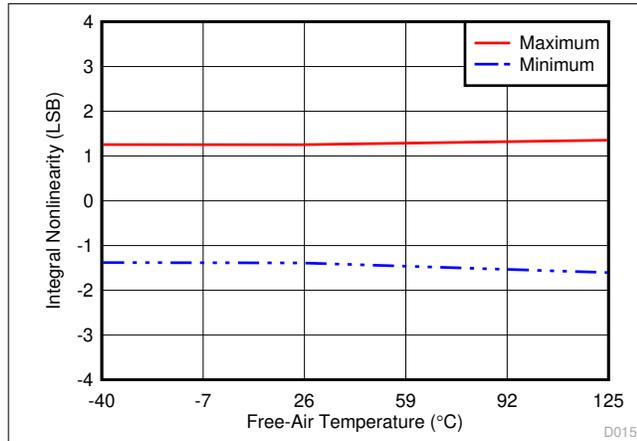
Figure 6-27. INL vs Temperature (All Unipolar Ranges)
