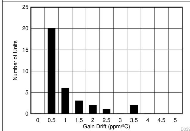
Figure 6-31. Typical Histogram for Gain Error Drift
