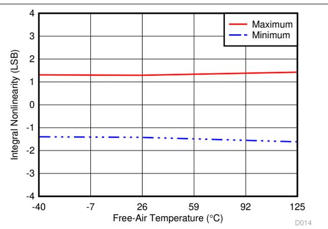
**Figure 6-26. INL vs Temperature (All Bipolar Ranges)**
