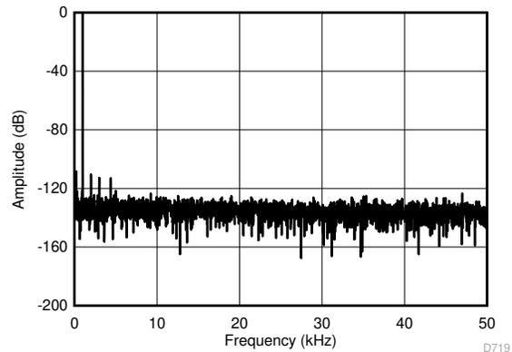
$f_{\text{SAMPLE}} = 100 \text{ kSPS}$ ,  $V_{\text{IN}} = \pm 12 \text{ V}$ ,  $f_{\text{IN}} = 1 \text{ kHz}$ ,  $V_{\text{CM}} = 155 \text{ V}_{\text{PP}}$ ,
