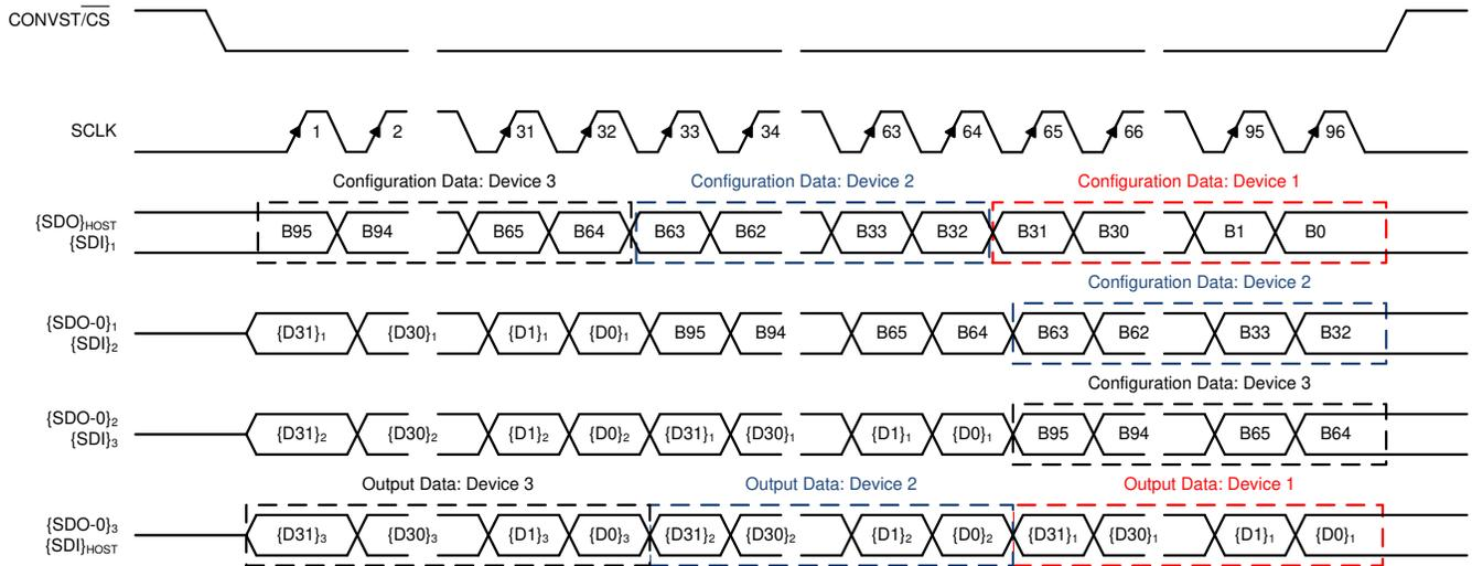
**Figure 7-23. Three Devices in Daisy-Chain Mode Timing Diagram**
