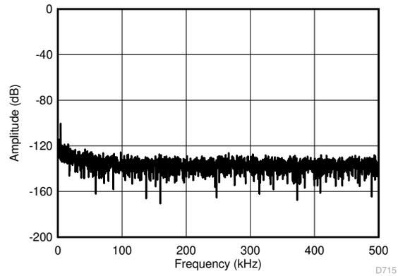
$f_{\text{SAMPLE}} = 1 \text{ MspS}$ ,  $V_{\text{IN}} = \pm 12 \text{ V}$ ,  $f_{\text{IN}} = 1 \text{ kHz}$ ,  $V_{\text{CM}} = 155 \text{ V}_{\text{PP}}$ ,
