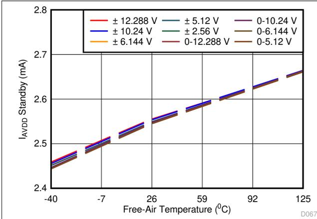
Figure 6-45. AVDD Current vs Temperature (Standby Mode)
