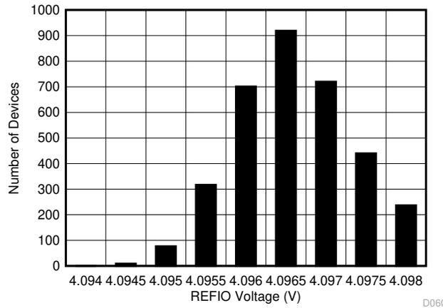
**Figure 7-8. Internal Reference Accuracy Histogram at Room Temperature**
