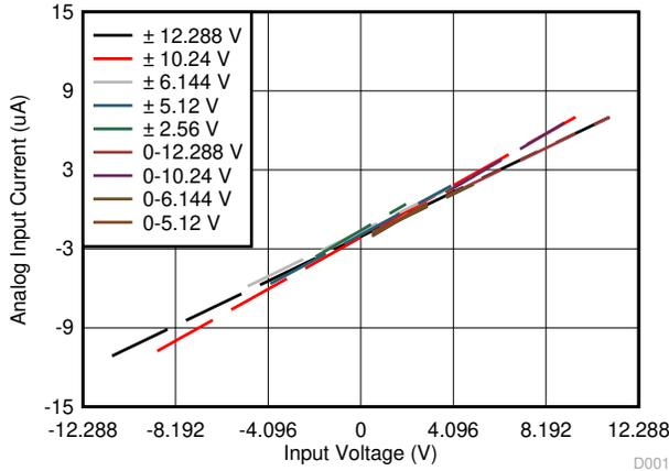
Figure 6-9. Input I-V Characteristic Across Input Ranges
