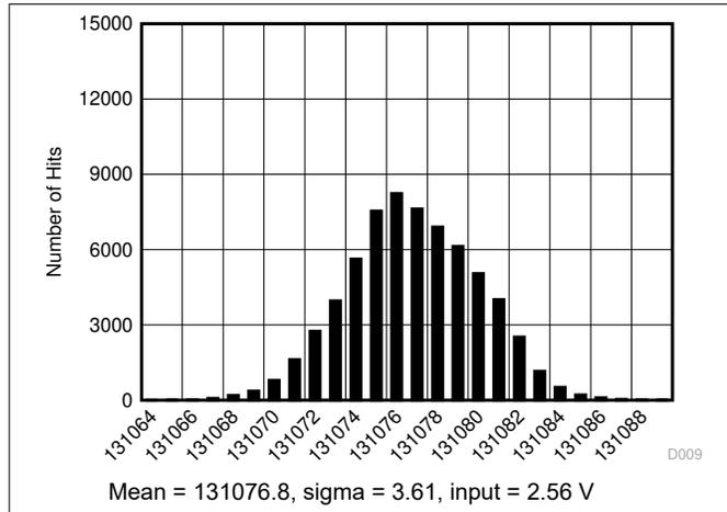
**Figure 6-21. DC Histogram for Mid-Scale Inputs (0 V–5.12 V)**
