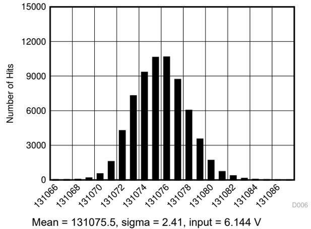
Figure 6-18. DC Histogram for Mid-Scale Inputs (0 V–12.288 V)
