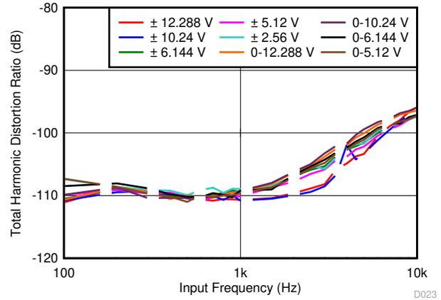
Figure 6-40. THD vs Input Frequency
