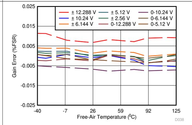
Figure 6-30. Gain Error vs Temperature Across Input Ranges
