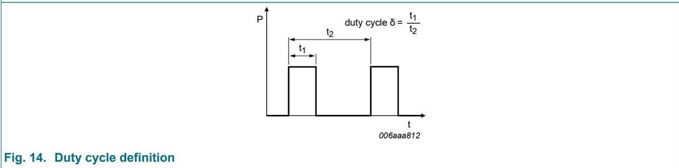
Fig. 14. Duty cycle definition
