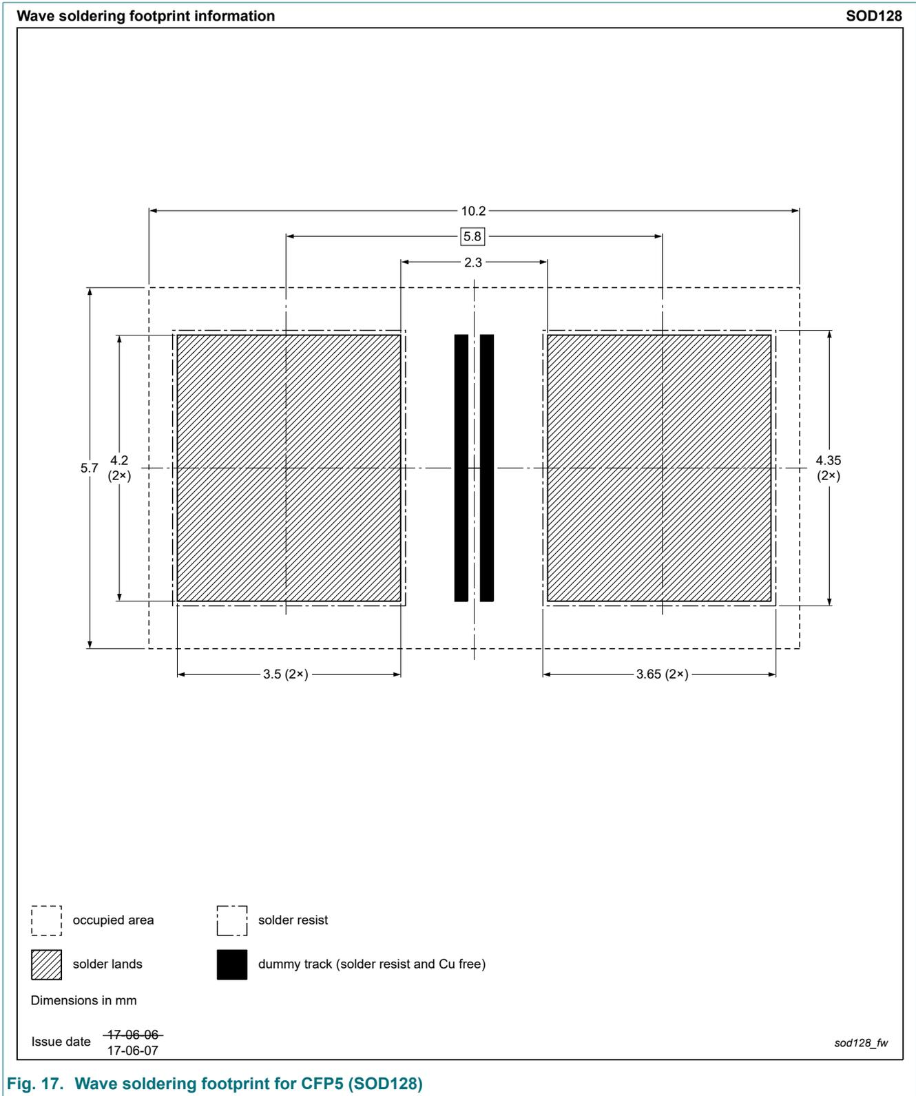
**Fig. 17. Wave soldering footprint for CFP5 (SOD128)**
