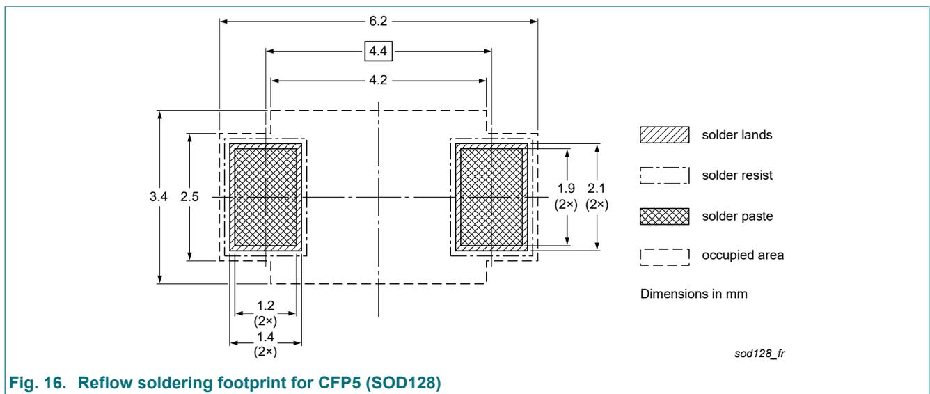
Fig. 16. Reflow soldering footprint for CFP5 (SOD128)
