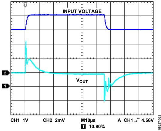
Figure 25. Line Transient Response,  $C_{IN}, C_{OUT} = 1 \mu F, I_{LOAD} = 200 mA$
