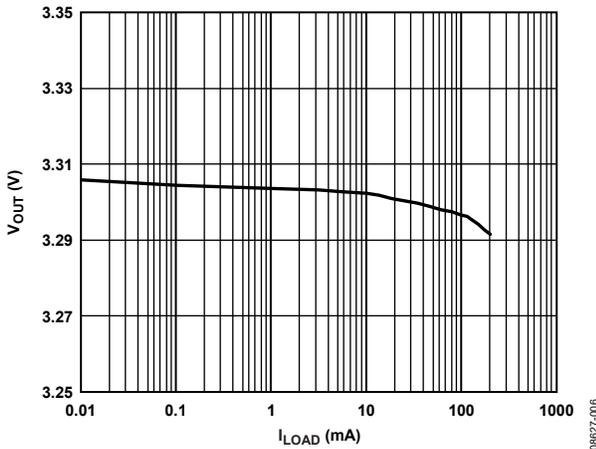
Figure 8.  $V_{OUT}$  vs. Load Current ( $I_{LOAD}$ )
