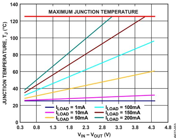
Figure 53. LFCSP 50 mm<sup>2</sup> of PCB Copper,  $T_A = 25^\circ\text{C}$
