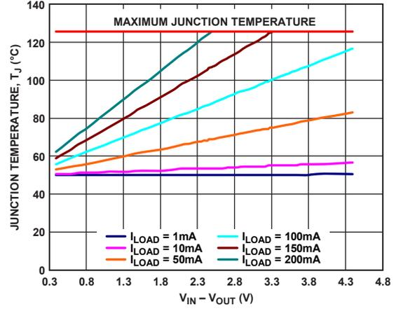
Figure 42. WLCSP 500 mm<sup>2</sup> of PCB Copper,  $T_A = 50^\circ\text{C}$
