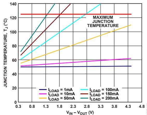
Figure 56. LFCSP 50 mm<sup>2</sup> of PCB Copper,  $T_A = 50^\circ\text{C}$
