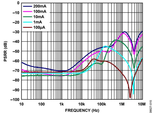
Figure 17. PSRR vs. Frequency, VOUT = 1.2 V, VIN = 2.2 V
