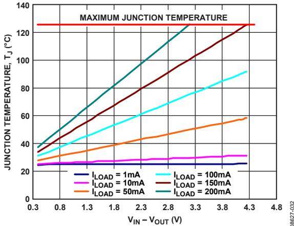
Figure 40. WLCSP 100 mm<sup>2</sup> of PCB Copper,  $T_A = 25^\circ\text{C}$
