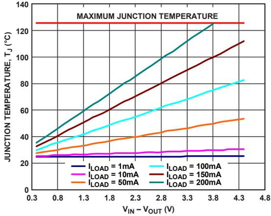
Figure 45. TSOT 500 mm<sup>2</sup> of PCB Copper, T<sub>A</sub> = 25°C
