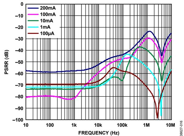
Figure 18. PSRR vs. Frequency, VOUT = 2.8 V, VIN = 3.3 V
