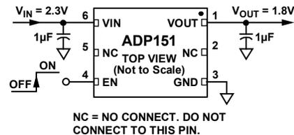
Figure 3. LFCSP ADP151 with Fixed Output Voltage, 1.8 V
