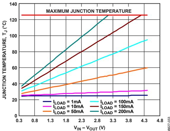
Figure 41. WLCSP 50 mm<sup>2</sup> of PCB Copper,  $T_A = 25^\circ\text{C}$
