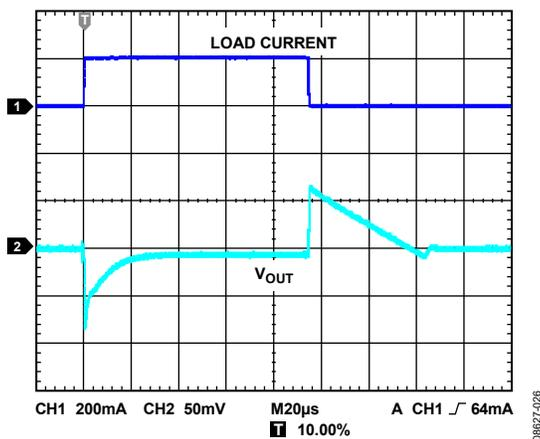
Figure 28. Output Transient Response,  $C_{OUT} = 1 \mu\text{F}$
