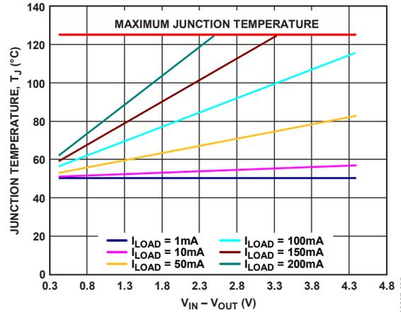
Figure 54. LFCSP 500 mm<sup>2</sup> of PCB Copper,  $T_A = 50^\circ\text{C}$
