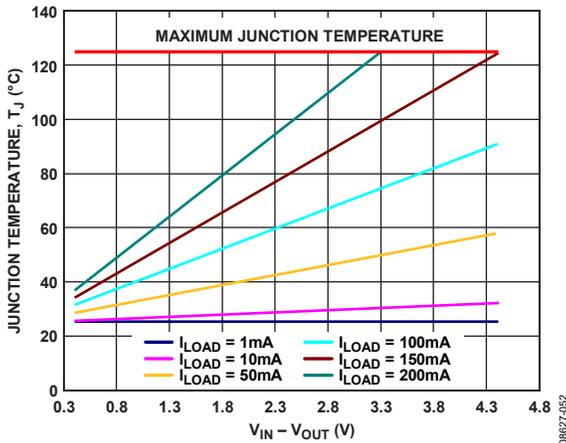
Figure 52. LFCSP 100 mm<sup>2</sup> of PCB Copper,  $T_A = 25^\circ\text{C}$
