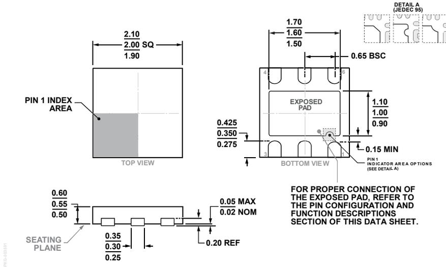
Figure 65. 6-Lead Lead Frame Chip Scale Package [LFCSP],
