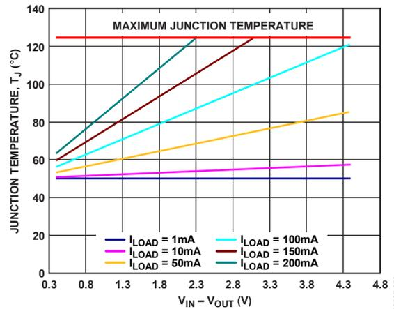
Figure 55. LFCSP 100 mm<sup>2</sup> of PCB Copper,  $T_A = 50^\circ\text{C}$
