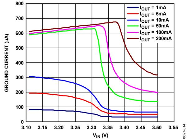
Figure 16. Ground Current vs. VIN (in Dropout)
