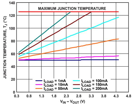
Figure 50. TSOT 50 mm<sup>2</sup> of PCB Copper, T<sub>A</sub> = 50°C
