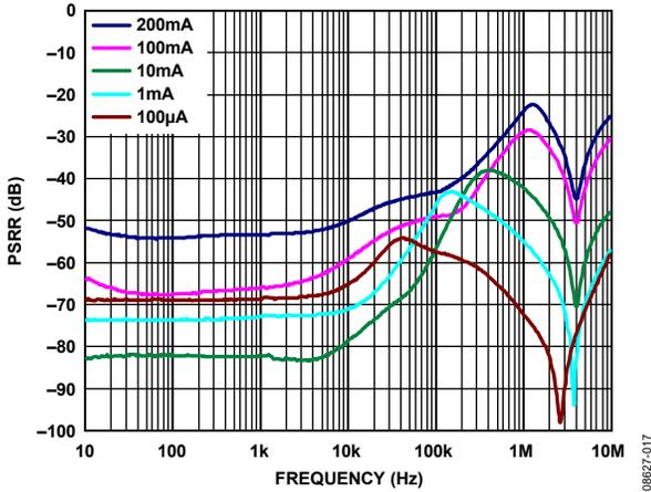
Figure 19. PSRR vs. Frequency,  $V_{OUT} = 3.3V$ ,  $V_{IN} = 3.8V$
