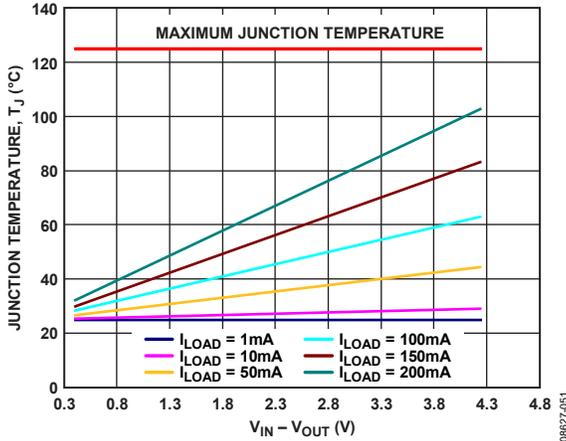
Figure 51. LFCSP 500 mm<sup>2</sup> of PCB Copper,  $T_A = 25^\circ\text{C}$
