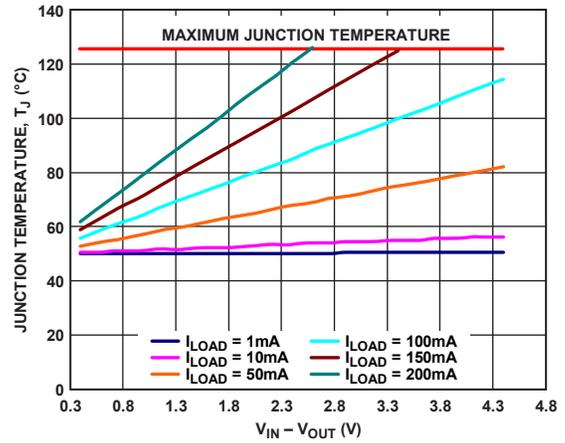
Figure 49. TSOT 100 mm<sup>2</sup> of PCB Copper, T<sub>A</sub> = 50°C
