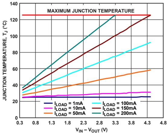
Figure 47. TSOT 50 mm<sup>2</sup> of PCB Copper, T<sub>A</sub> = 25°C
