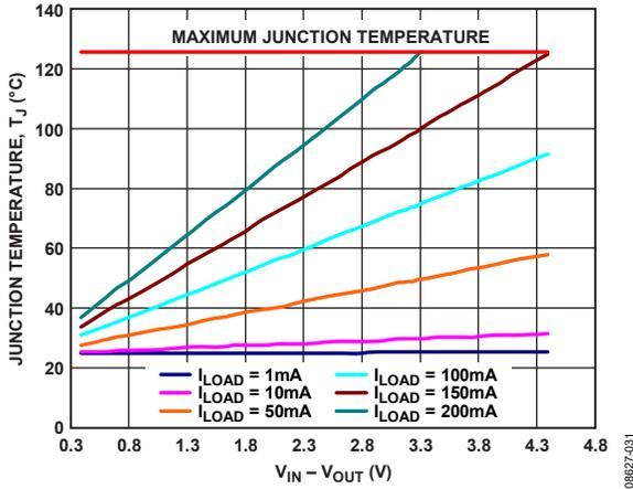
Figure 39. WLCSP 500 mm<sup>2</sup> of PCB Copper,  $T_A = 25^\circ\text{C}$
