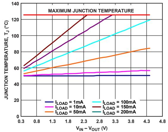
Figure 43. WLCSP 100 mm<sup>2</sup> of PCB Copper,  $T_A = 50^\circ\text{C}$
