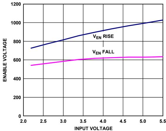
Figure 31. Typical EN Pin Thresholds vs. Input Voltage
