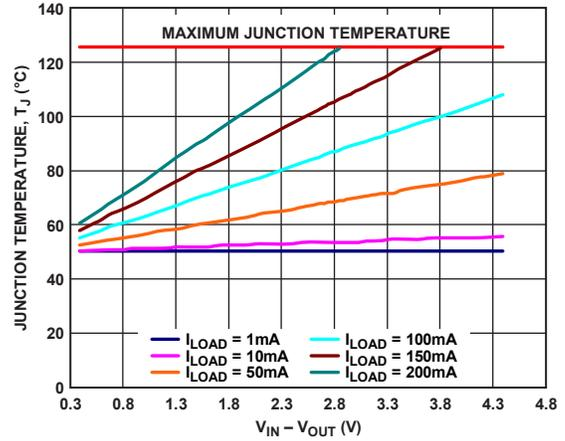
Figure 48. TSOT 500 mm<sup>2</sup> of PCB Copper, T<sub>A</sub> = 50°C
