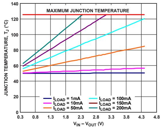
Figure 44. WLCSP 50 mm<sup>2</sup> of PCB Copper,  $T_A = 50^\circ\text{C}$
