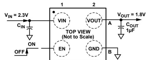
Figure 2. WLCSP ADP151 with Fixed Output Voltage, 1.8 V
