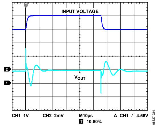
Figure 26. Line Transient Response,  $C_{IN}, C_{OUT} = 1 \mu F, I_{LOAD} = 1 mA$
