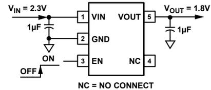
Figure 1. TSOT ADP151 with Fixed Output Voltage, 1.8 V
