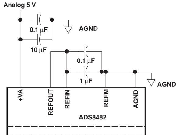
**Figure 36. ADS8482 Using Internal Reference**
