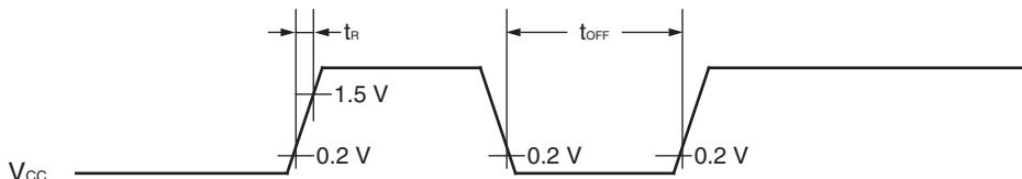
Note: A sudden change of power supply voltage may activate the power-on reset function. When changing the power supply voltage during the operation, set the slope of rising to a value below within 20 mV/ms as shown below.
