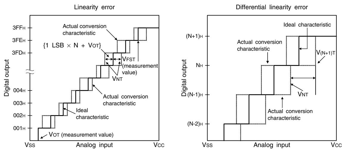
$$\text{Linearity error of digital output } N = \frac{V_{NT} - \{1 \text{ LSB} \times N + V_{OT}\}}{1 \text{ LSB}}$$
