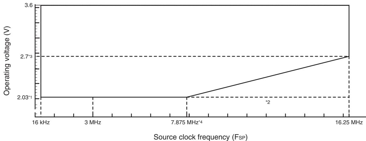
\*1: This is the default LVD reset clear threshold:  $1.93\text{ V} \pm 0.10\text{ V}$ . It can also be set to  $2.40\text{ V} \pm 0.15\text{ V}$  or  $2.95\text{ V} \pm 0.15\text{ V}$ .
