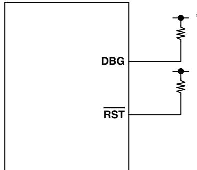
\*: Since the DBG input pin becomes a communication pin in on-chip debug mode, set a pull-up resistor value suiting the input/output specifications of P12/DBG.
