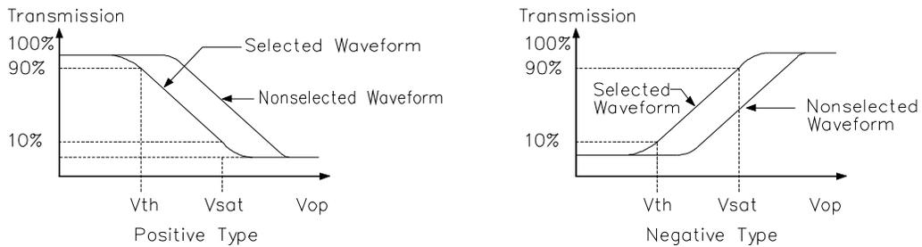
**Vth:** The voltage Vop which the transmission rate of segment is 90%(positive) or 10%(negative) of saturated value on conditions of the selected waveform.(non-selected waveform is opposition)
