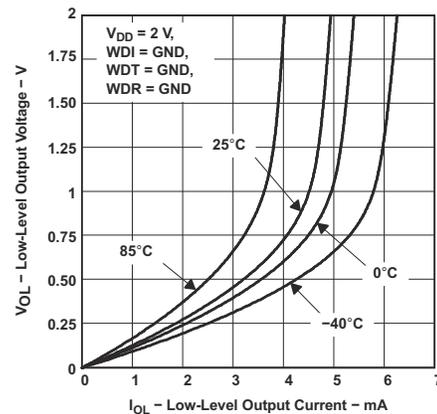
Figure 7-3. Low-Level Output Voltage vs Low-Level Output Current
