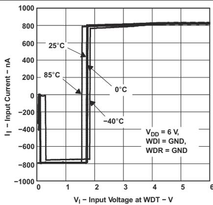
Figure 7-4. Input Current vs Input Voltage at WDT
