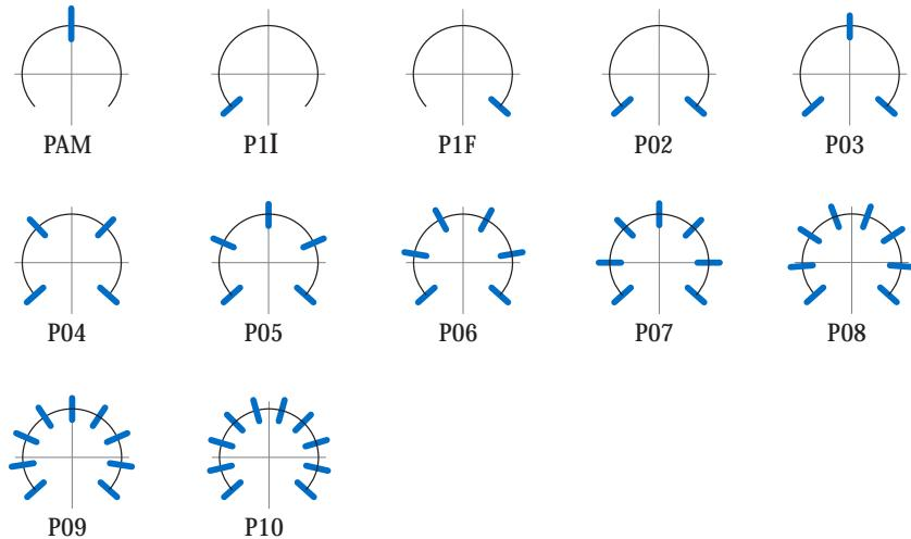
Relative detent positions along the total mechanical travel.
