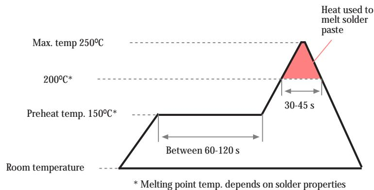
This recommended reflow profile is provided as a guideline. Optimal profile may differ due to oven type, assembly layout or other design or process variables. Customers should verify actual device performance in their specific application and reflow process. Please contact Piher if you require additional support.
