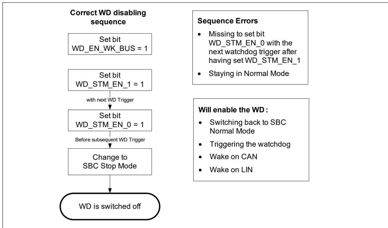
Figure 41 Watchdog Disabling Sequence (with wake via BUS)
