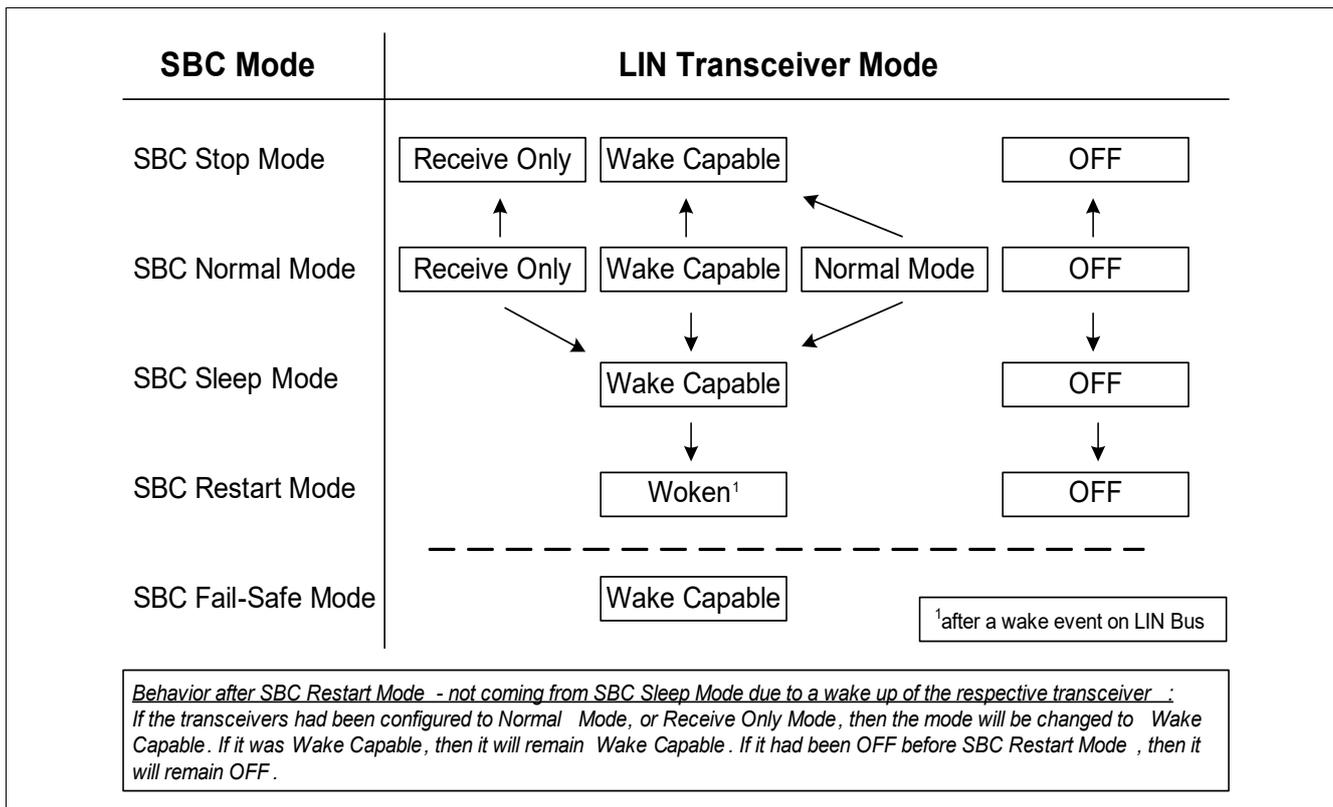
**Figure 24 LIN Mode Control Diagram**
