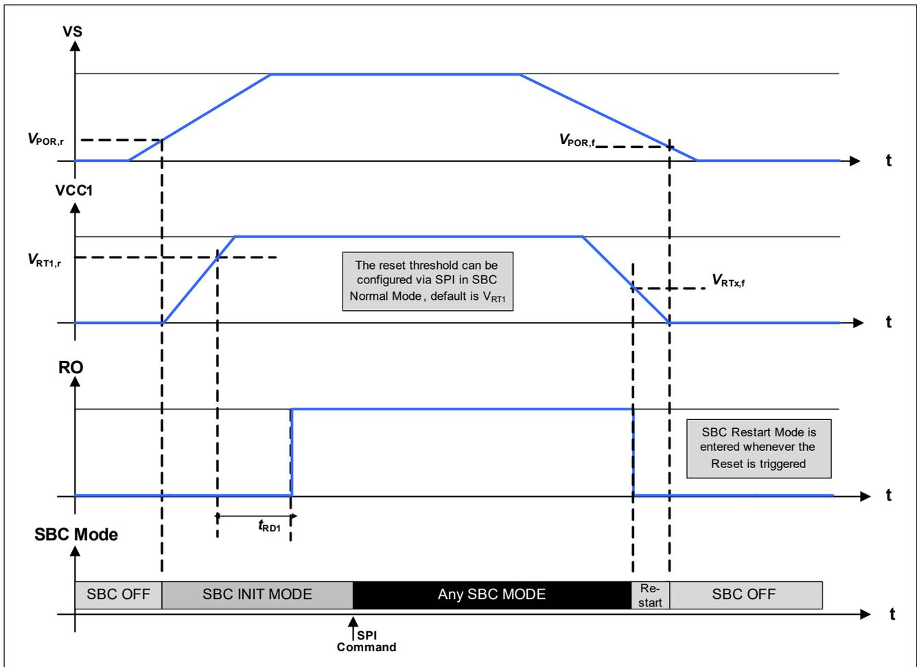
Figure 42 Ramp up / down example of Supply Voltage
