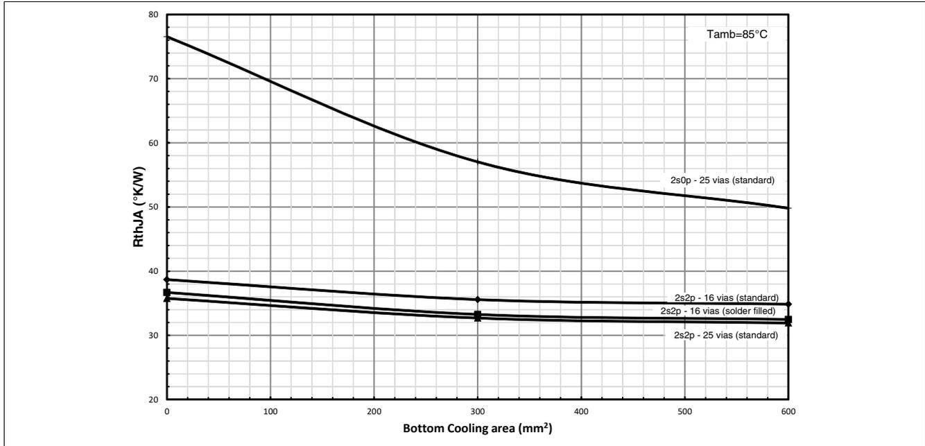
Figure 53 Thermal Resistance ( $R_{th\_JA}$ ) vs. Cooling Area
