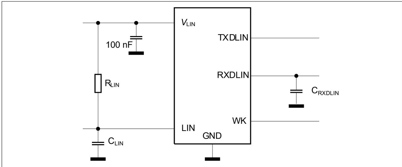
**Figure 27** Simplified Test Circuit for Dynamic Characteristics
