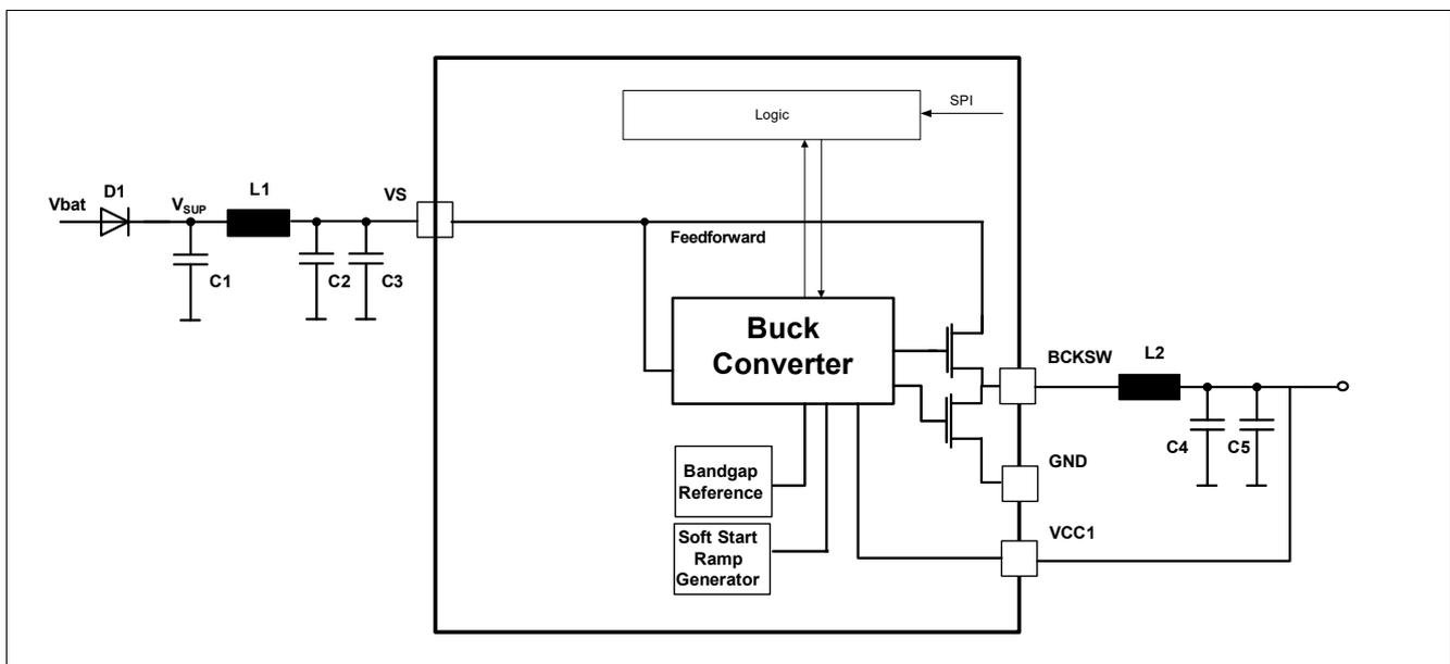
**Figure 7 Buck Block Diagram**
