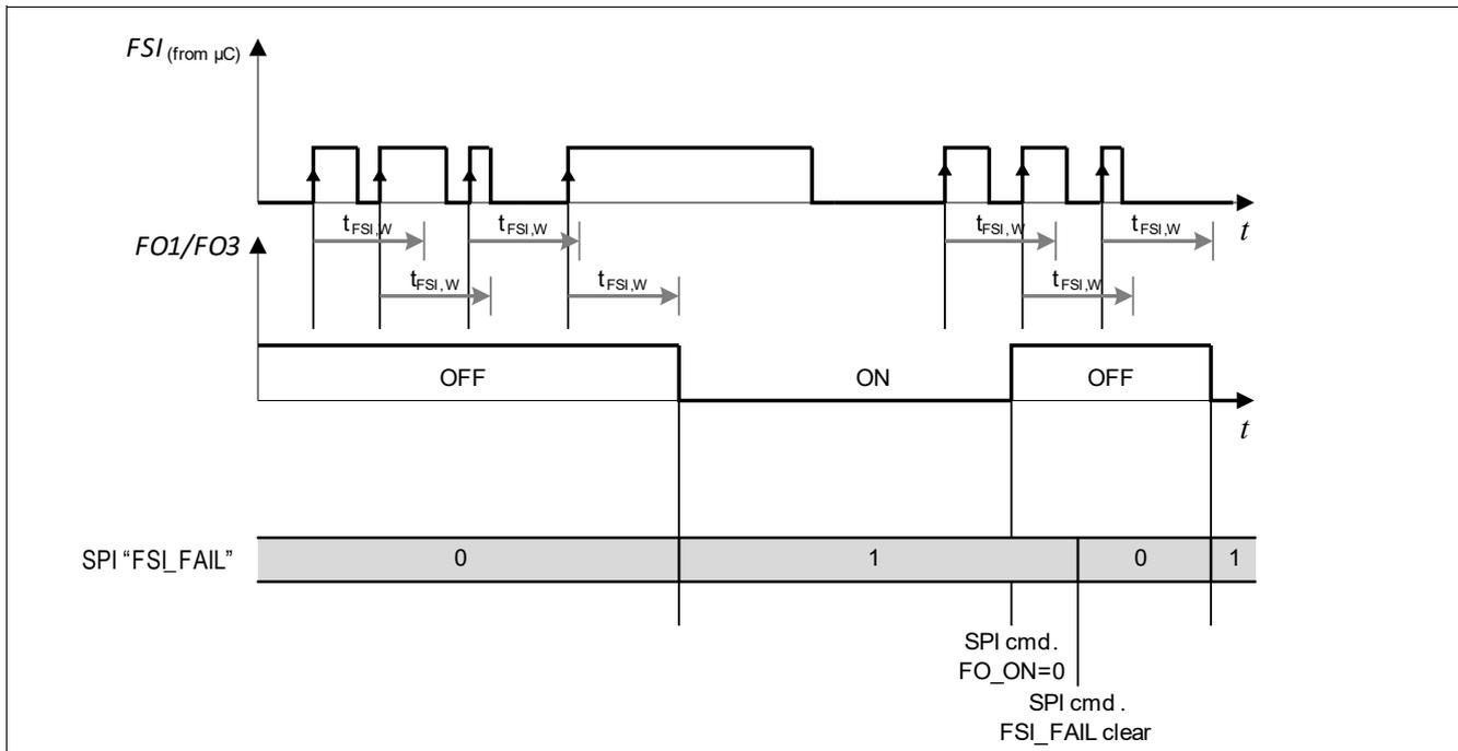
**Figure 35 FSI timing diagram and level description**
