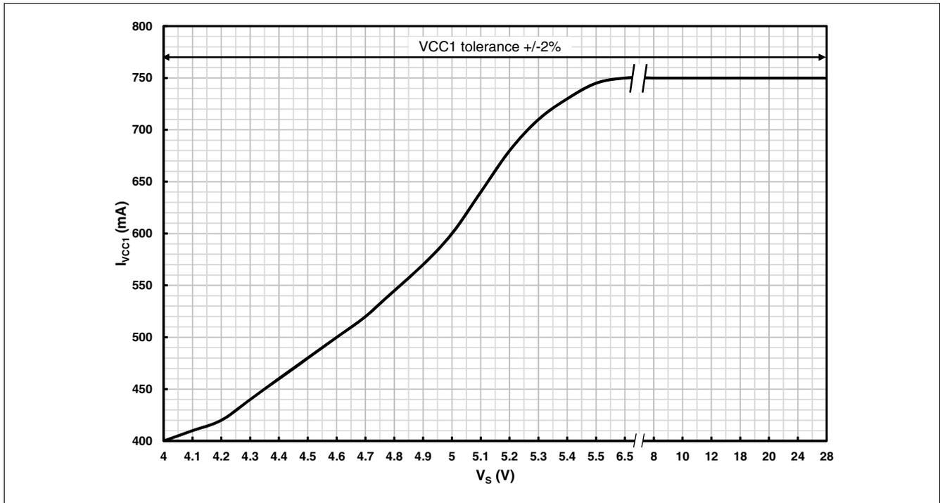
Figure 12 Maximum DCDC Buck current capability versus VS.
