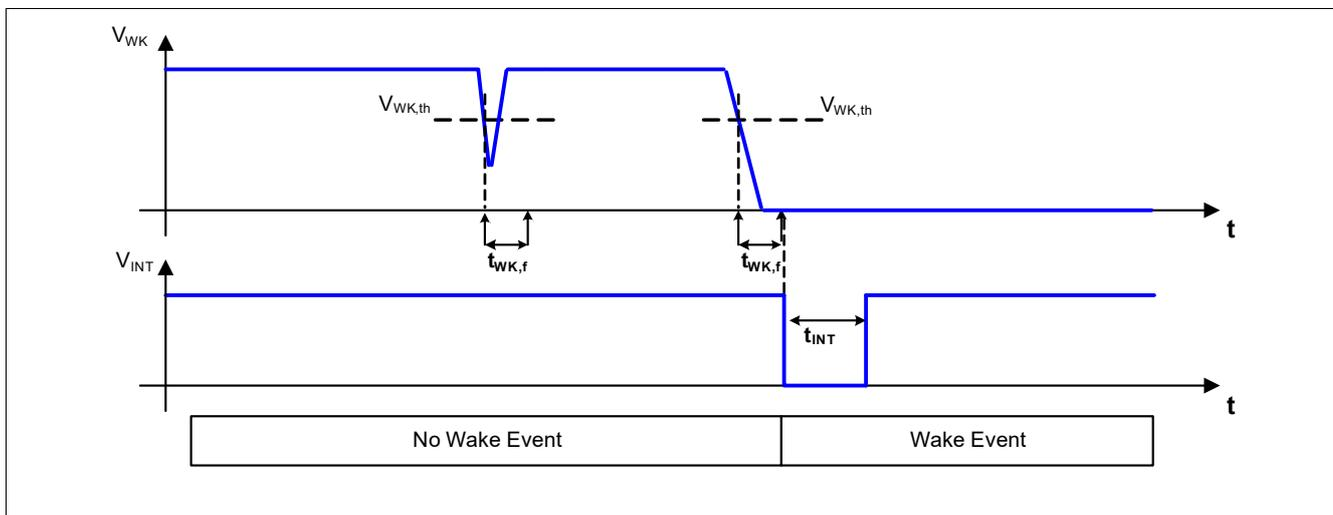
**Figure 30** Wake-up Filter Timing for Static Sense
