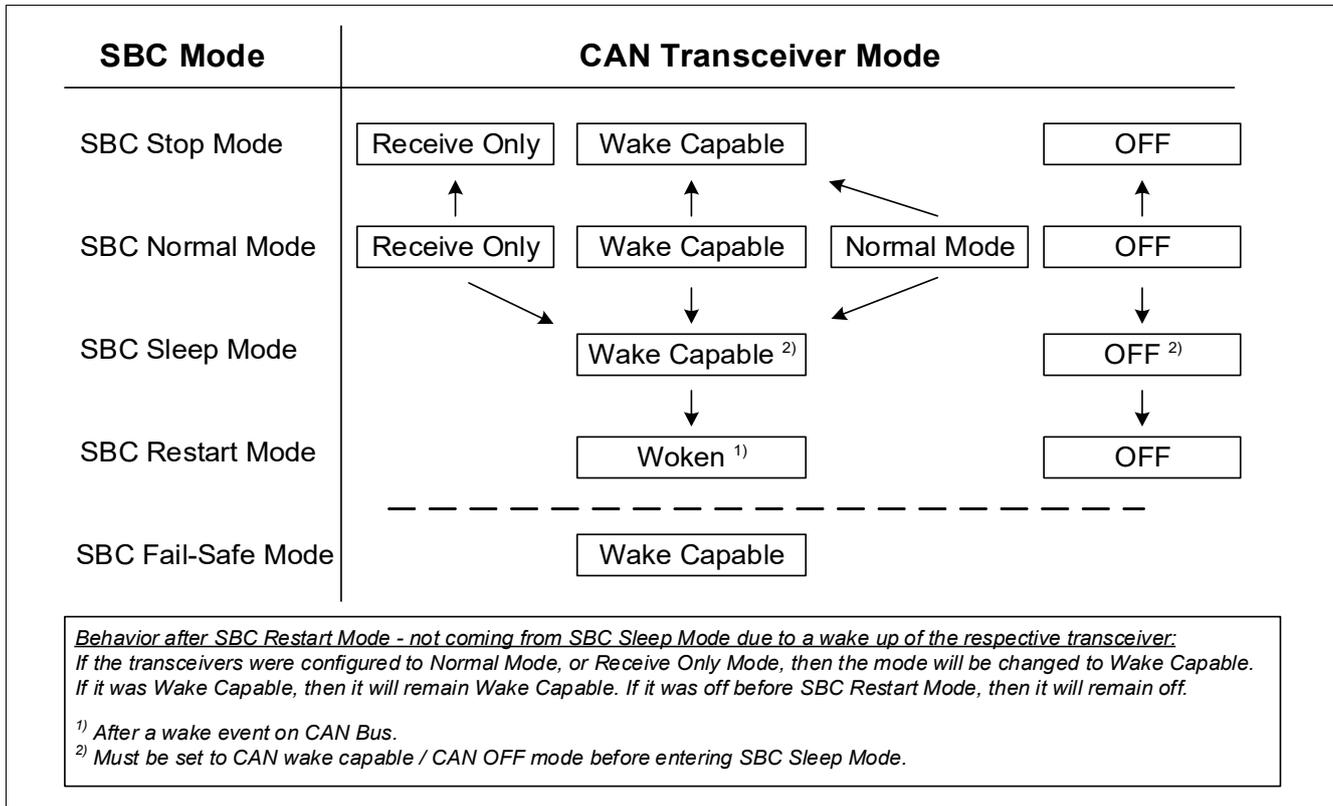
Figure 17 CAN Mode Control Diagram
