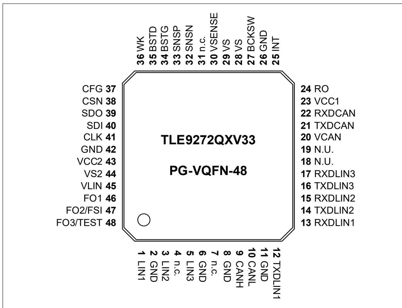
**Figure 2 Pin Configuration**
