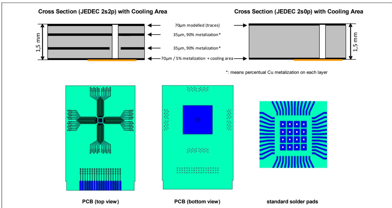
Figure 54 Board Setup
