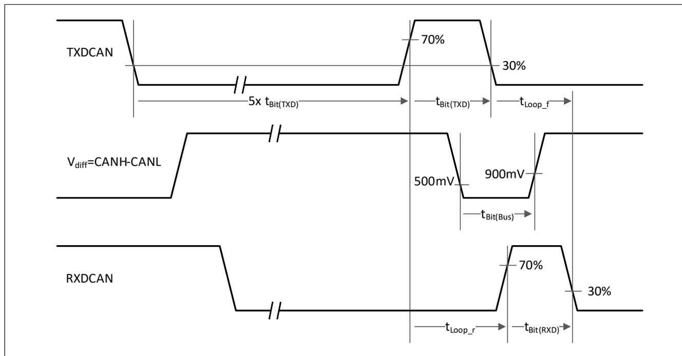
Figure 22 From ISO 11898-2: t<sub>loop</sub>, t<sub>bit(TXD)</sub>, t<sub>bit(Bus)</sub>, t<sub>bit(RXD)</sub> Definitions
