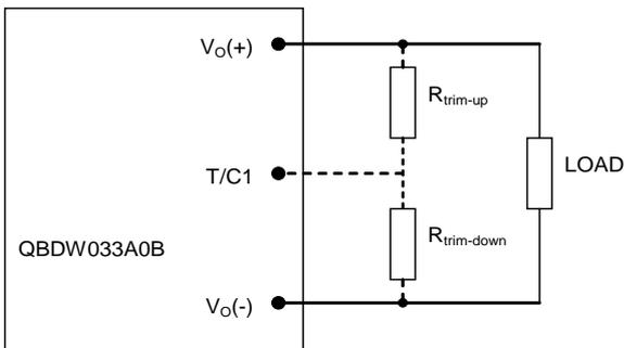
**Figure 16. Circuit Configuration to Trim Output Voltage.**
