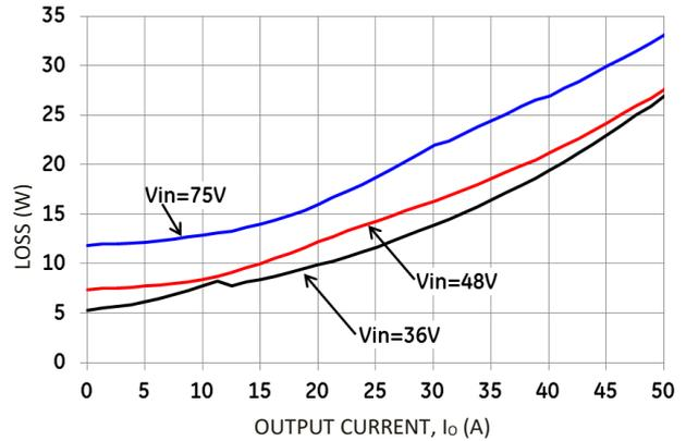
Figure 2. Typical Converter Loss vs. Output Current.
