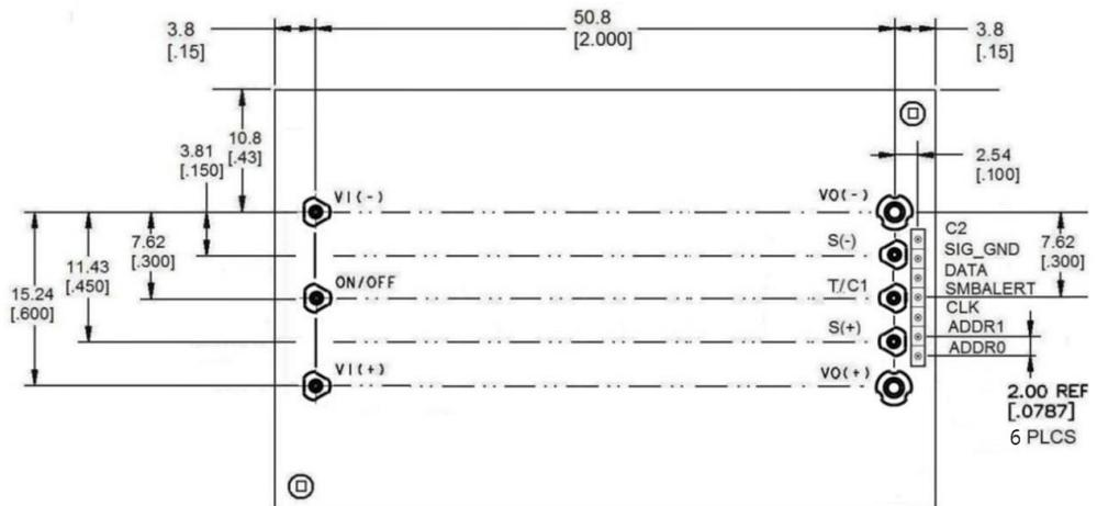
**QSD(V)W050A0B Barracuda Series; DC-DC Converter Power Modules**
