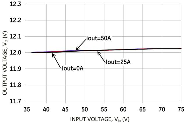
Figure 7. Typical Output Voltage Regulation vs. Input Voltage.
