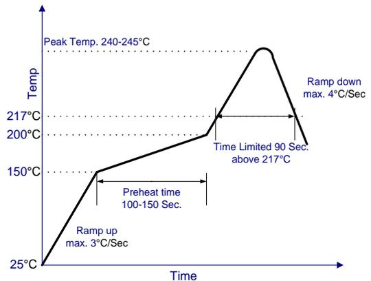
**Figure 24. Recommended linear reflow profile using Sn/Ag/Cu solder.**
