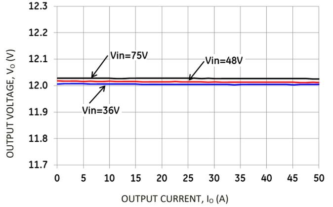
Figure 8. Typical Output Voltage Regulation vs. Output Current.
