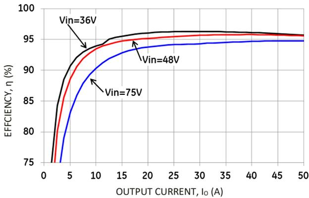
Figure 1. Typical Converter Efficiency vs. Output Current.
