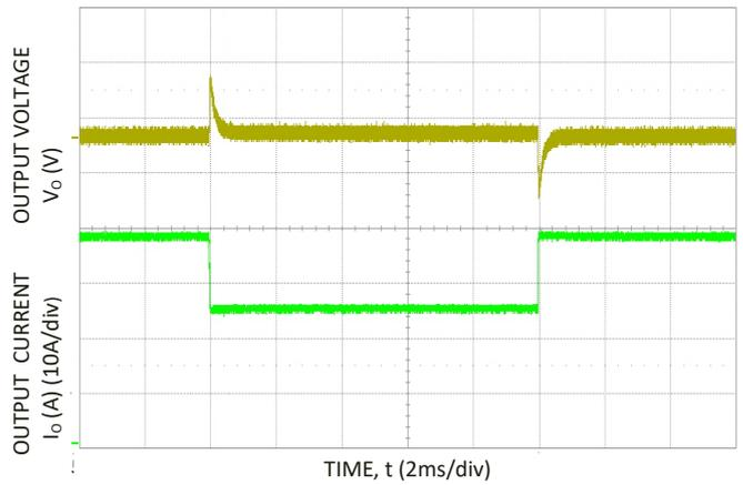
Figure 4. Typical Transient Response to 1.0A/µs Step Change in Load from 50% to 75% to 50% of Full Load,  $C_o = 470\mu F$  and 48 Vdc Input.
