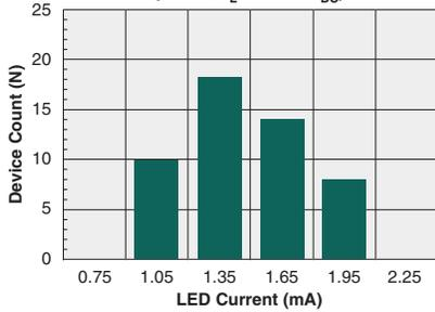
**Typical  $I_F$  for Switch Dropout**
