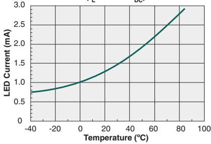
**Typical  $I_F$  for Switch Dropout vs. Temperature**
