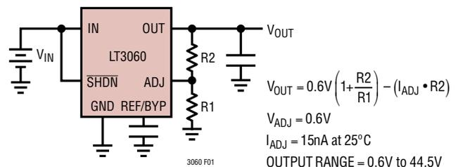
Figure 1. Adjustable Operation
