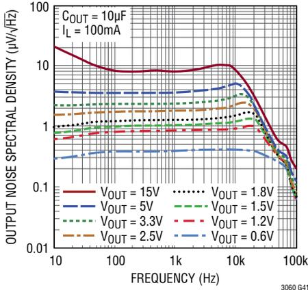
**Output Noise Spectral Density vs  $C_{\text{REF/BYP}}, C_{\text{FF}} = 0$**
