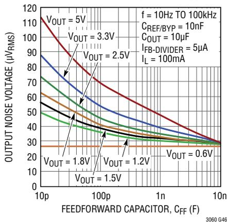
**RMS Output Noise vs Feedforward Capacitor ( $C_{\text{FF}}$ )**
