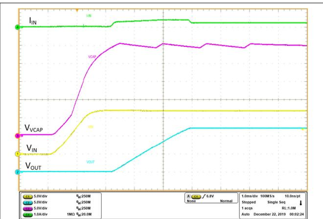
Figure 10-3. Startup 12 V showing Charge Pump VCAP
