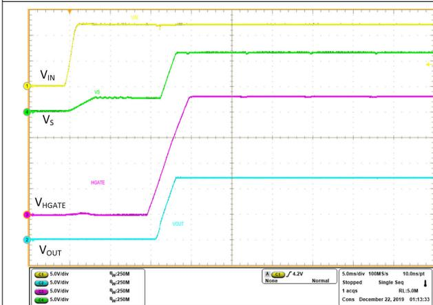
**Figure 10-25. Power up 12 V - HGATE and Output**
