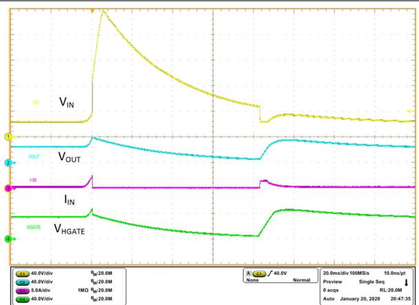
**Figure 10-22. Unsuppressed Load Dump 200 V - Output Cut-off**
