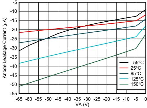
Figure 7-7. ANODE Leakage Current vs Reverse ANODE Voltage
