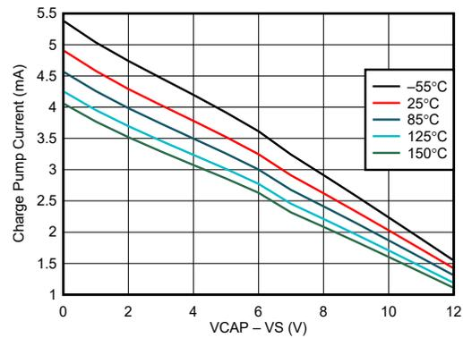
Figure 7-4. Charge Pump V-I Characteristics at VS ≥ 12 V
