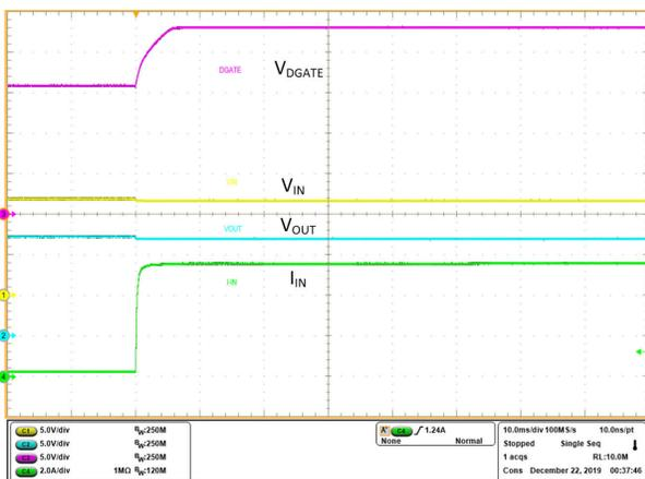
Figure 10-18. Load Transient 100 mA to 5 A
