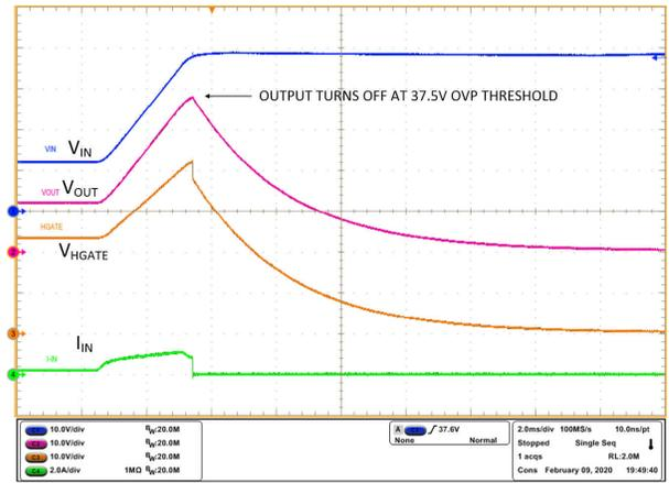
**Figure 10-13. Overvoltage Protection**
