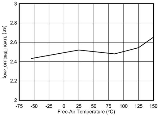
Figure 7-13. HGATE Turn OFF Delay During OV
