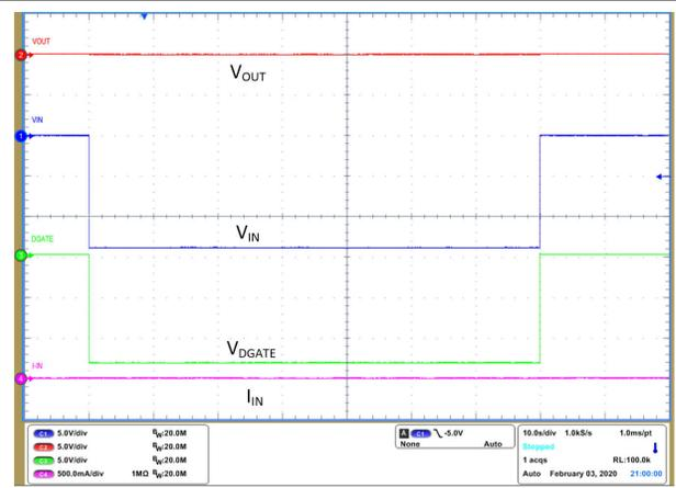
Figure 10-5. Reverse Input Voltage -14 V for 60 s
