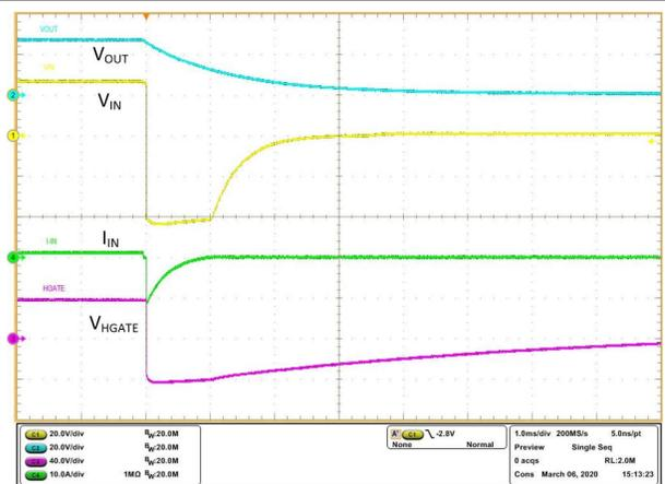
**Figure 10-24. ISO 7637-2 Pulse 1 –600 V 50 Ω**
