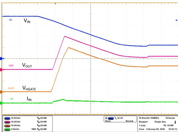
**Figure 10-14. Overvoltage Recovery**
