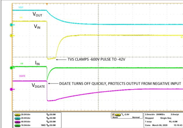
**Figure 10-23. ISO 7637-2 Pulse 1 –600 V 50 Ω**
