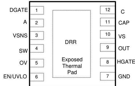
Figure 6-1. DRR Package, 12-Pin WSON (Top View)
