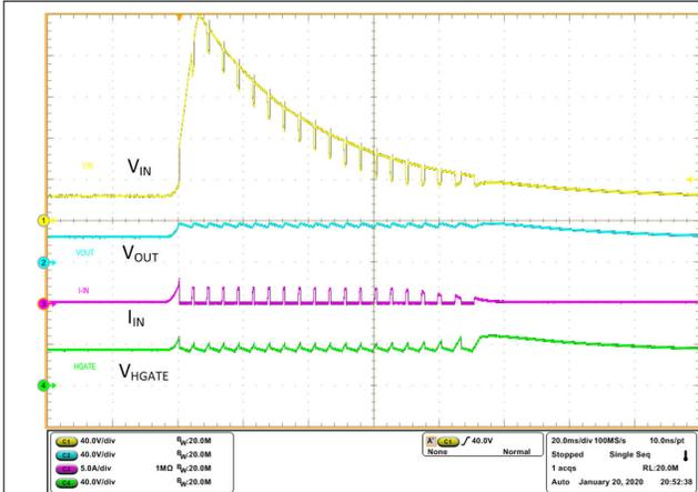
**Figure 10-21. Unsuppressed Load Dump 200 V - Output Clamp**
