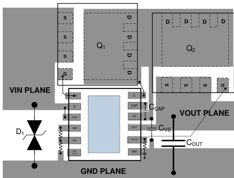
Figure 10-30. PCB Layout Example for Common Drain Configuration
