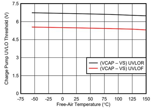
Figure 7-10. Charge Pump UVLO Threshold vs Temperature
