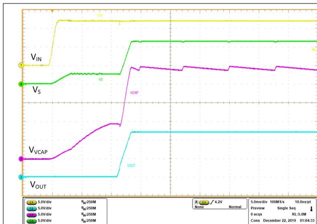
**Figure 10-27. Power up 12 V - Charge Pump VCAP**
