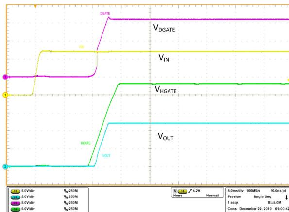
**Figure 10-28. Power up 12 V - DGATE and HGATE**
