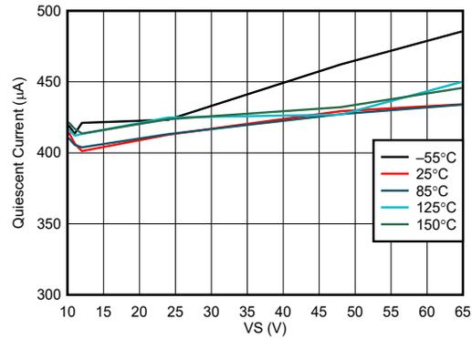
Figure 7-2. Operating Quiescent Current vs Supply Voltage (> 10 V)
