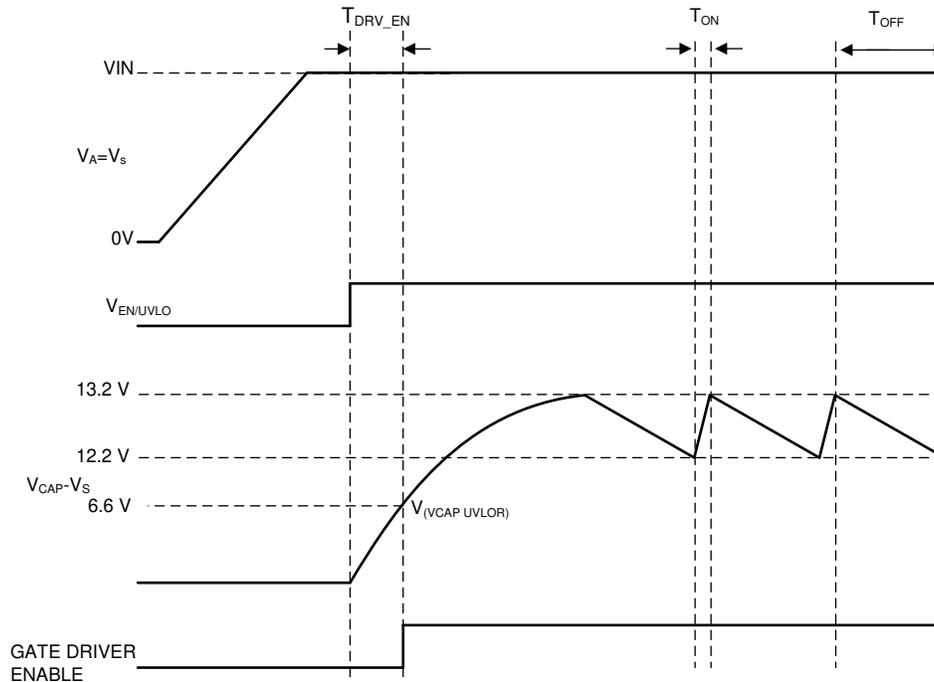
**Figure 9-1. Charge Pump Operation**
