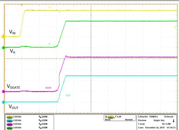
**Figure 10-26. Power up 12 V - DGATE and A**
