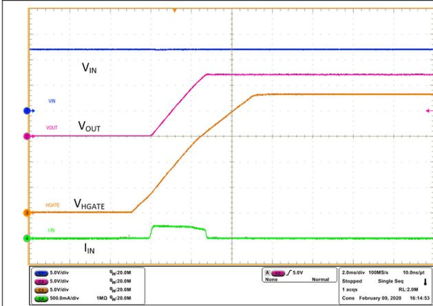
Figure 10-6. Inrush Current with no Load at Output
