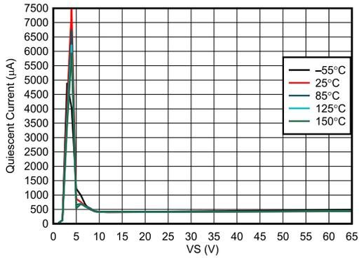
Figure 7-1. Operating Quiescent Current vs Supply Voltage
