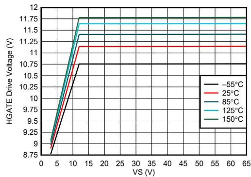
Figure 7-6. HGATE Drive Voltage vs Supply Voltage
