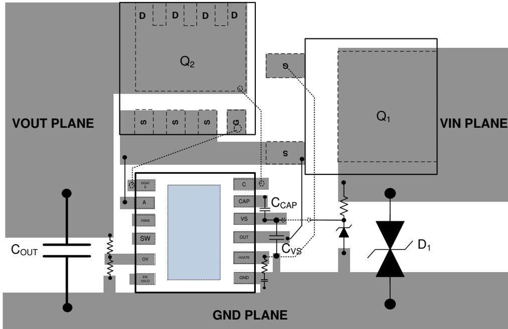
Figure 10-31. PCB Layout Example for Common Source Configuration
