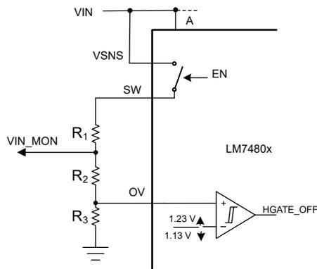
**Figure 9-4. Programming Overvoltage Threshold and Battery Sensing**
