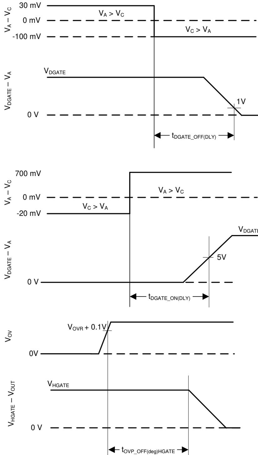
**Figure 8-1. Timing Waveforms**
