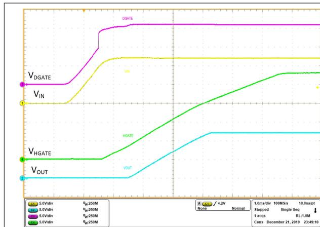
Figure 10-2. Startup 12 V with EN Pulled to VIN
