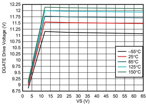
Figure 7-5. DGATE Drive Voltage vs Supply Voltage
