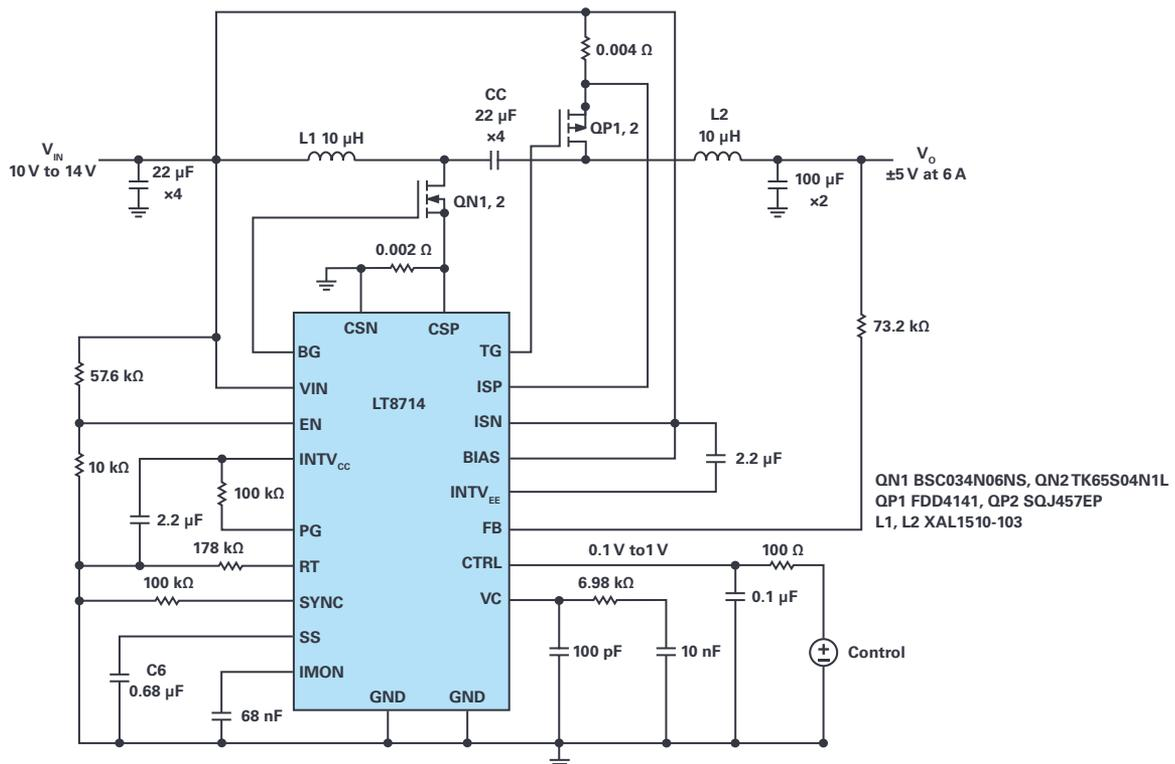
Figure 1. An electrical schematic of a power supply based on the LT8714 operating in two quadrants  $V_{IN}$  12 V,  $V_O$   $\pm 5$  V at 6 A.
