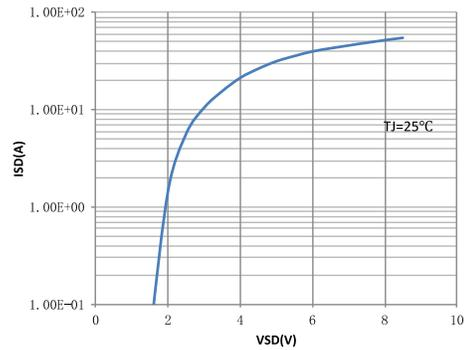
$I_{sd}$  vs.  $V_{sd}$  reverse conduction curve @ 25 °C
