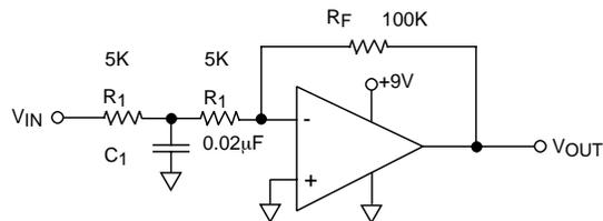
$$\text{Cutoff frequency} = \frac{1}{\pi R_1 C_1} = 3.2KHz$$
