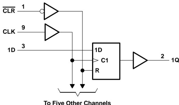
Pin numbers shown are for the D, DB, DGV, J, N, NS, PW, and W packages.
