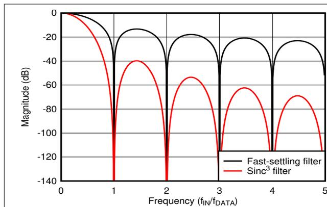
**Figure 8-5. Fast-Settling and Sinc<sup>3</sup> Digital Filter Response**
