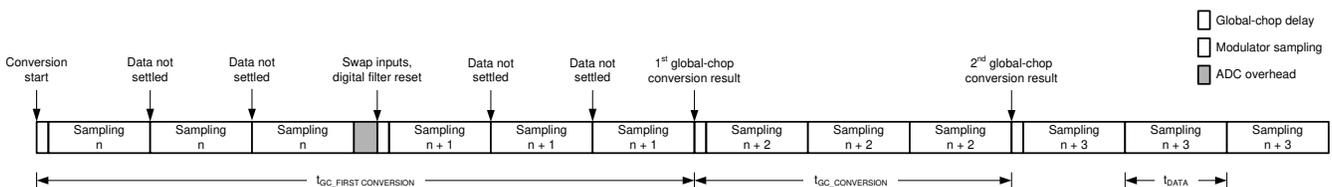
Figure 8-12. Conversion Timing With Global-Chop Mode Enabled
