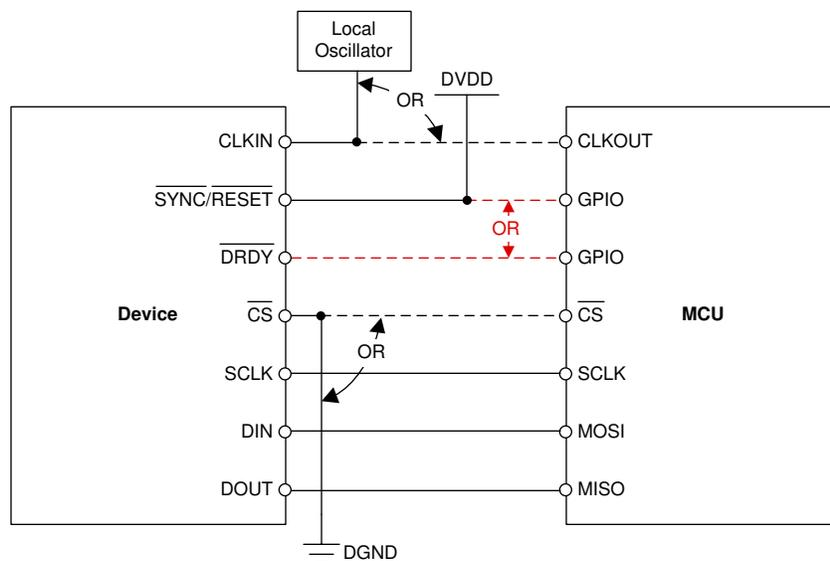
**Figure 9-2. Minimum Connections Required to Operate the ADS130B04-Q1**
