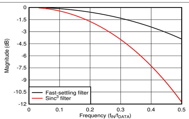
**Figure 8-6. Fast-Settling and Sinc<sup>3</sup> Digital Filter Response, Pass-Band Detail**
