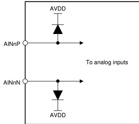
**Figure 8-1. Input ESD Protection Circuitry**
