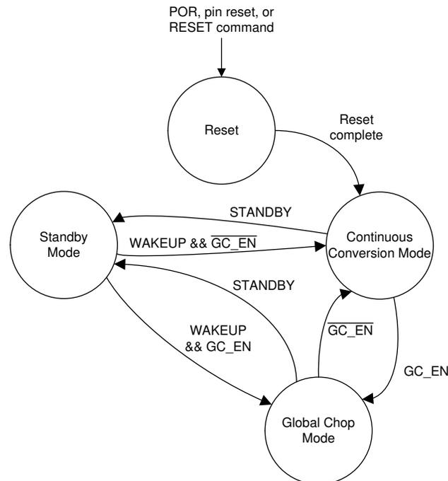
Figure 8-9. State Diagram Depicting Device Functional Modes
