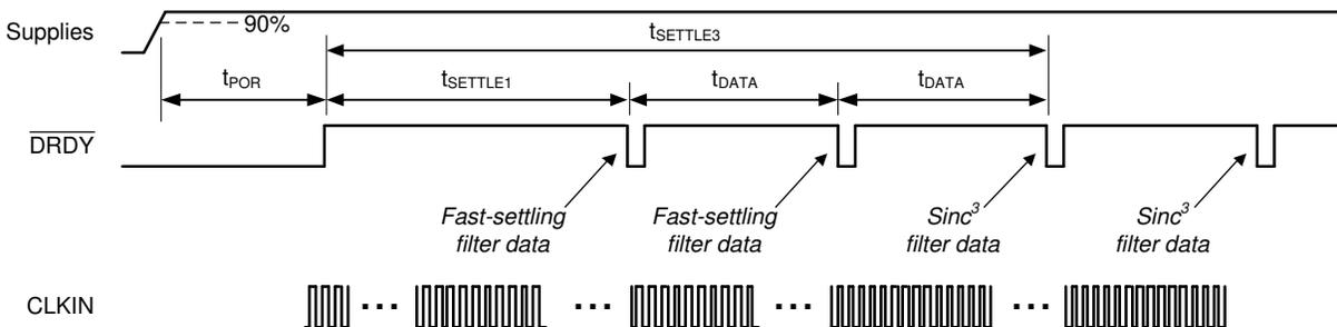
Figure 8-10. Fast Start-Up Behavior and Settling Times
