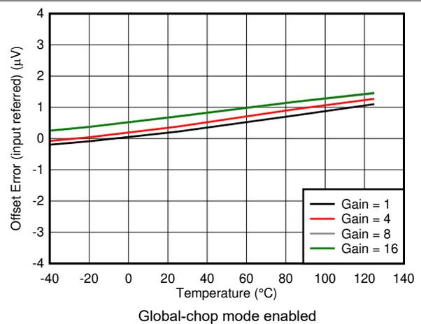
Figure 6-7. Offset Error vs Temperature
