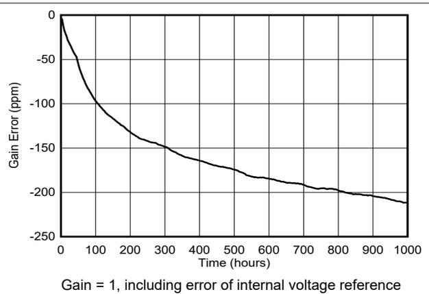
Figure 6-9. Gain Error Long-Term Drift
