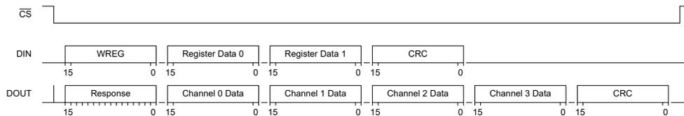
Figure 8-14. SPI Frame using 16-bit Word Size
