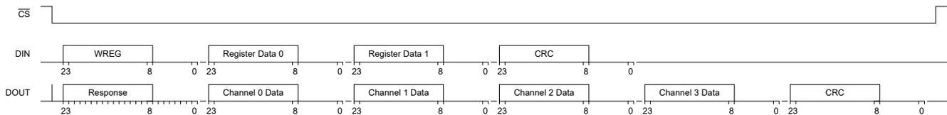
Figure 8-15. SPI Frame using 24-bit, zero-padded Word Size
