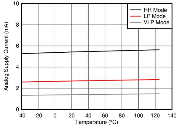
Gain = 1, OSR = 1024, all four ADC channels enabled
