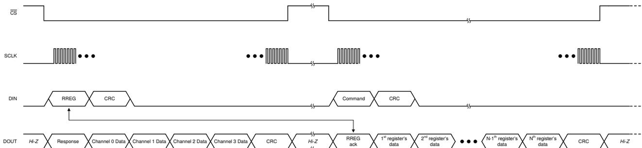
Figure 8-20. Reading Multiple Registers
