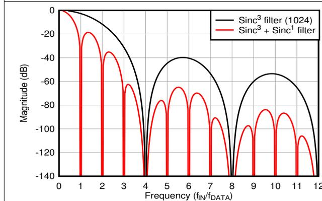
**Figure 8-7. Digital Filter Response for OSR = 1024 and OSR = 4096**
