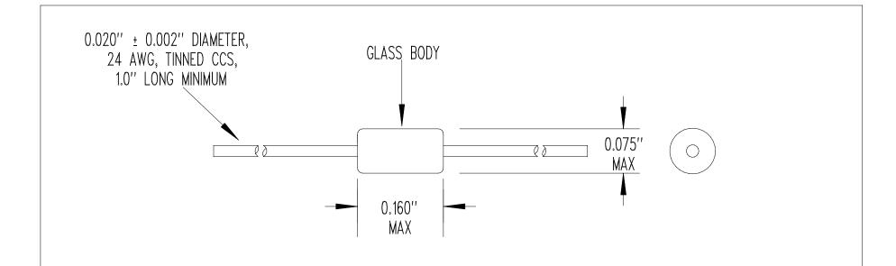
RESISTANCE @  $+25^{\circ}C = 2,500 \Omega \pm 5\%$ RESISTANCE/TEMPERATURE CURVE = "F" BETA " $\beta$ " (0 TO  $+50^{\circ}C$ ) = 3,419 $^{\circ}K$  NOMINAL TEMPERATURE COEFFICIENT @  $+25^{\circ}C = -3.86\%/^{\circ}C$  NOMINAL DISSIPATION CONSTANT = 2 mW/ $^{\circ}C$  NOMINAL (STILL AIR) THERMAL TIME CONSTANT = 5 SECONDS NOMINAL (STILL AIR) THERMAL TIME CONSTANT = 0.5 SECONDS NOMINAL (STIRRED OIL) MAXIMUM TEMPERATURE RATING =  $+300^{\circ}C$
