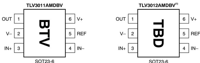
Note: Pin 1 is determined by orienting package marking as shown.
