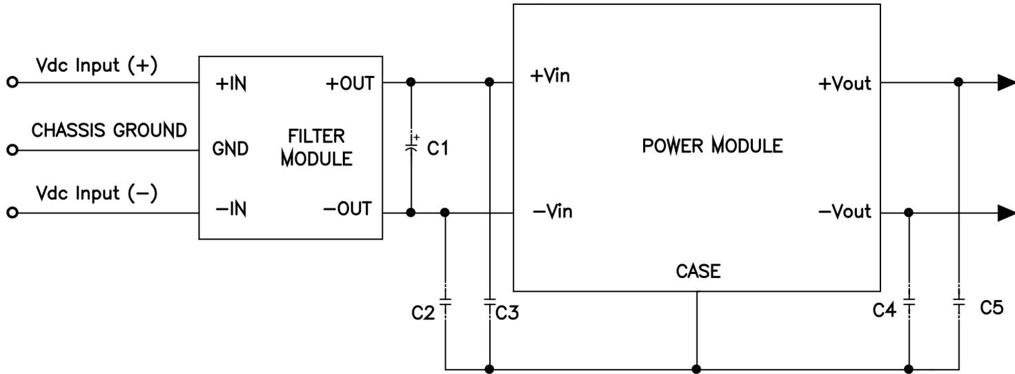
Note: C2 through C5 can be 0.01 $\mu$ F to 0.1 $\mu$ F. Select the voltage rating to meet input-to-output isolation requirements. C1 should be the recommended value suggested in the power module data sheet.
