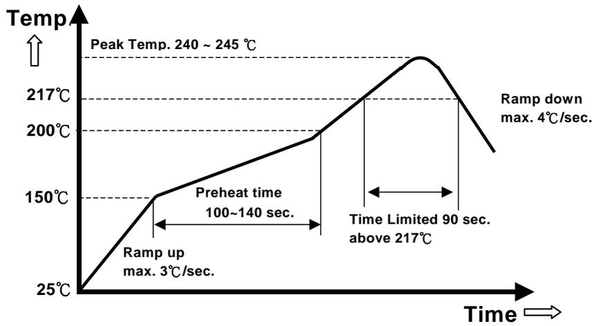
*Note: The temperature refers to the pin of filter 7A, measured on the pin 1 (+Vout) joint.*
