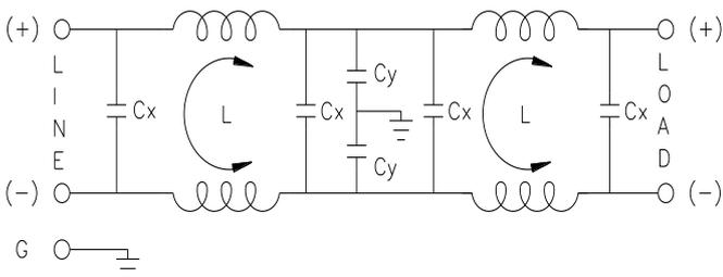
Figure 3: Internal schematics
