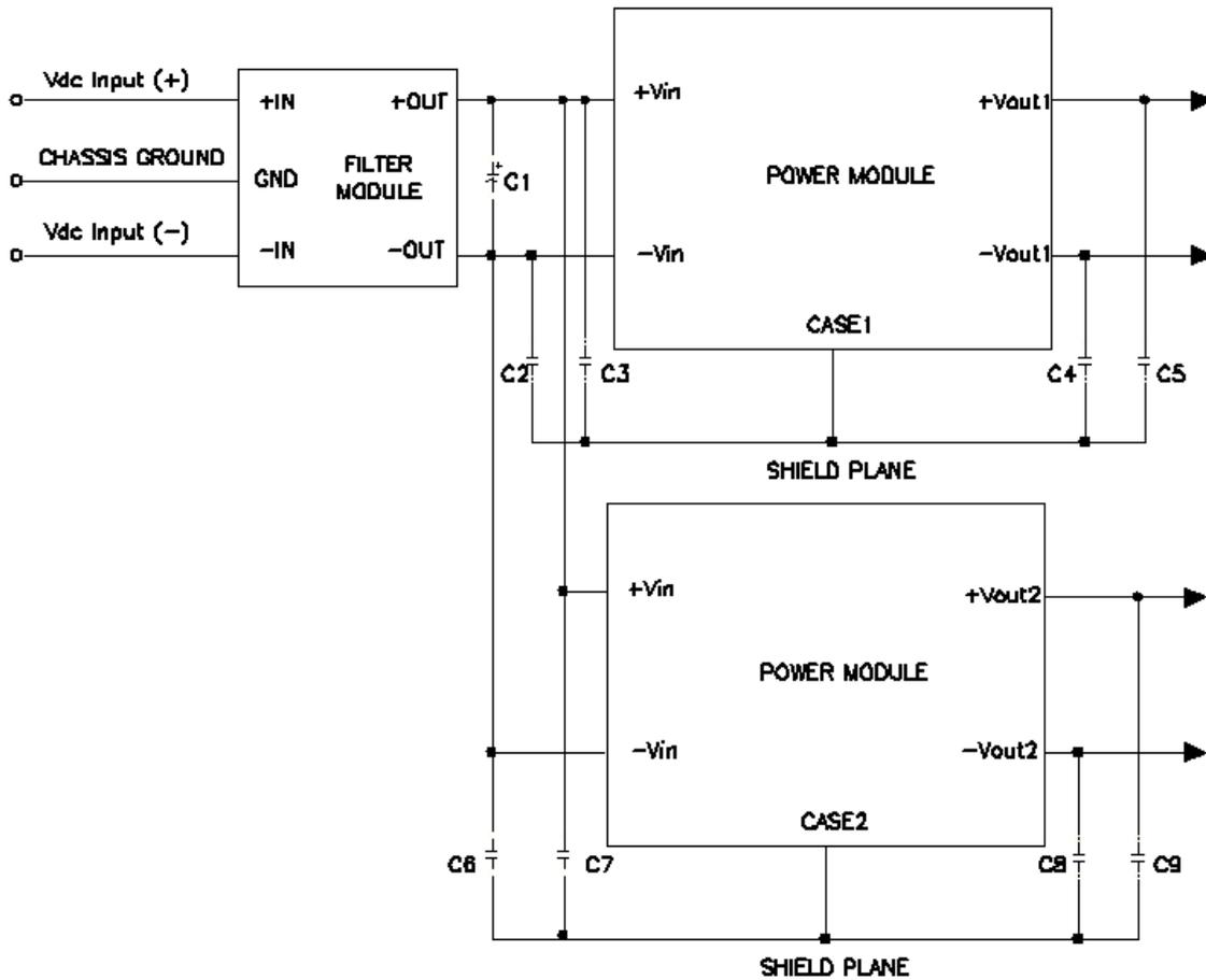
Note: : C2 through C5 and C6 through C9 can be 0.01 $\mu$ F to 0.1 $\mu$ F. Select the voltage rating to meet input-to-output isolation requirements. C1 should be the recommended value suggested in the power module datasheet.
