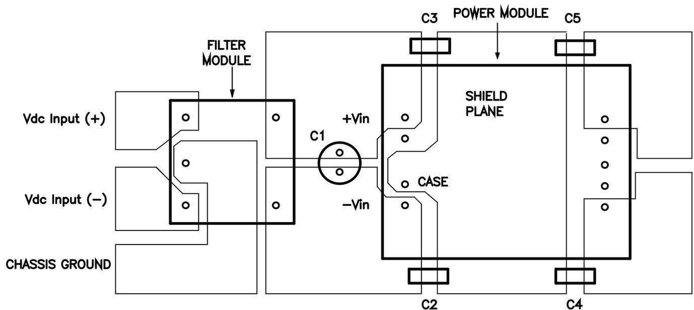
Note: Avoid routing signals or planes under the power module or the filter module. Please ensure all connections are low impedance.
