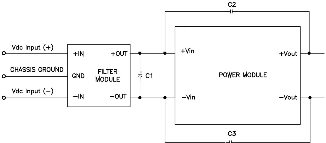
Note: C2 & C3 can be 0.01 $\mu$ F to 0.1 $\mu$ F. Select the voltage rating to meet input-to-output isolation requirements. C1 should be the recommended value suggested in the power module data sheet.
