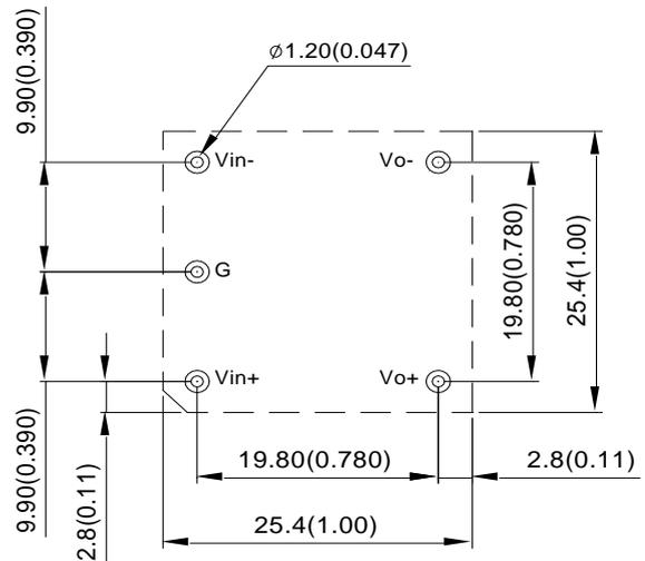
Note: Inside this filter module, the components have no voltage polarity. Hence, the input positive (Vin+) and input negative (Vin-) labels could be swapped for the convenience of layout and matching with power module input connected to the filter module, just remember to swap the output labels accordingly as well. Please refer to Figures 8 and 10 for how it is applied.
