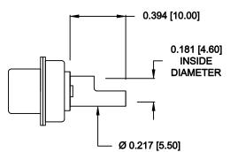
20 AMP POWER CONTACTS **ACCEPTS UP TO 12 AWG WIRE**
