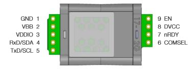
Figure 2 Pin configuration (Top view)
