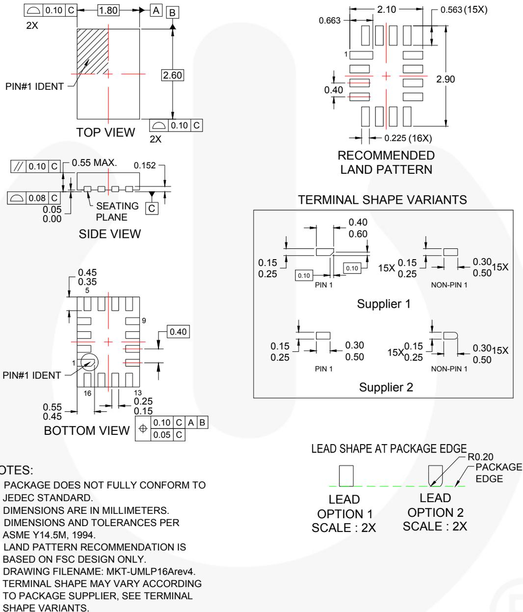
**Figure 10. 16-lead, UMLP, QUAD, Ultra-Thin MLP, 1.8 x 2.6 mm**
