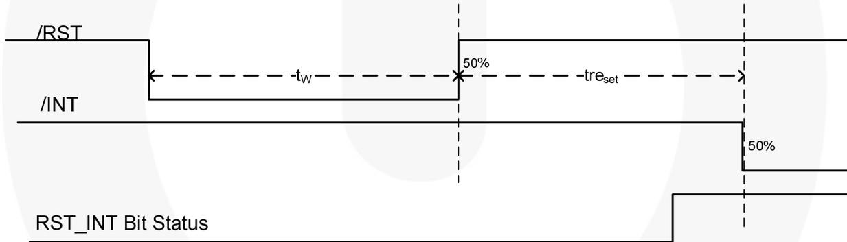
Figure 5. Reset Time and Reset Pulse Timing Diagram
