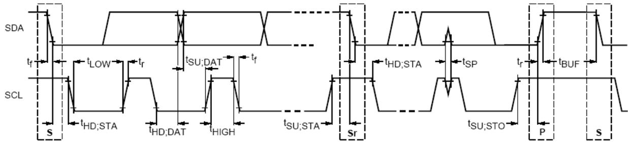
Figure 7. Definition of Timing for Full-Speed Mode Devices on the I<sup>2</sup>C-Bus<sup>®</sup>
