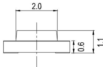
For reflow soldering (propose)
