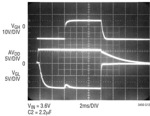
**AV<sub>DD</sub> Turn-On Showing Inrush Current Limiting**
