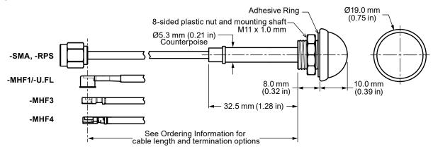
Figure 1. ANT-DB1-WRT Antenna Dimensions
