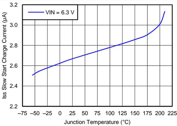
Figure 10. Slow Start Charge Current vs Temperature
