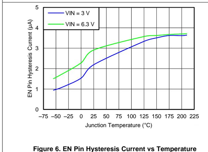
Figure 6. EN Pin Hysteresis Current vs Temperature
