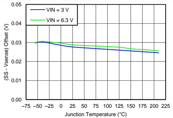
Figure 11. (SS - V<sub>SENSE</sub>) Offset vs Temperature
