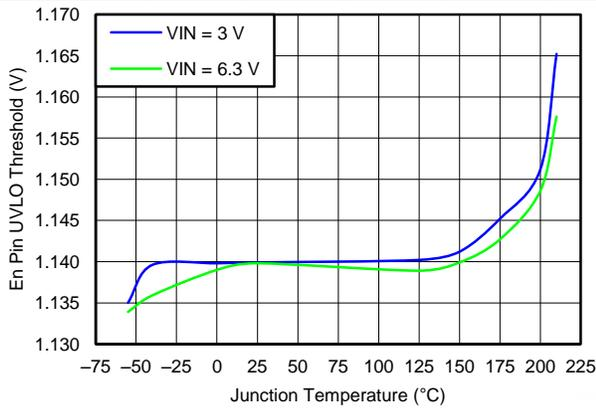
Figure 8. EN Pin UVLO Threshold vs Temperature
