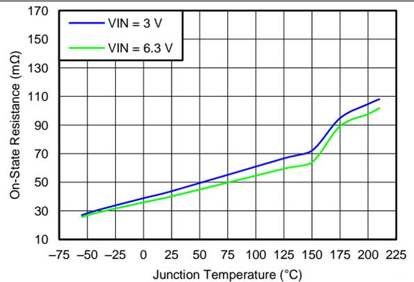
Figure 13. Low-Side R<sub>DS(on)</sub> vs Temperature
