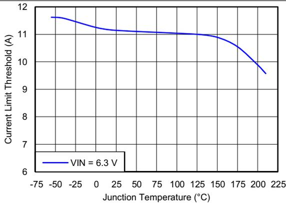
Figure 12. High-Side Current Limit Threshold vs Temperature
