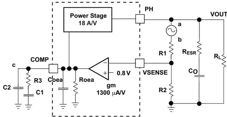
Figure 25. Small Signal Model For Loop Response
