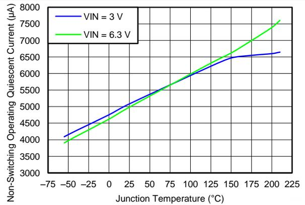
Figure 9. Non-Switching Operating Quiescent Current (VIN) vs Temperature
