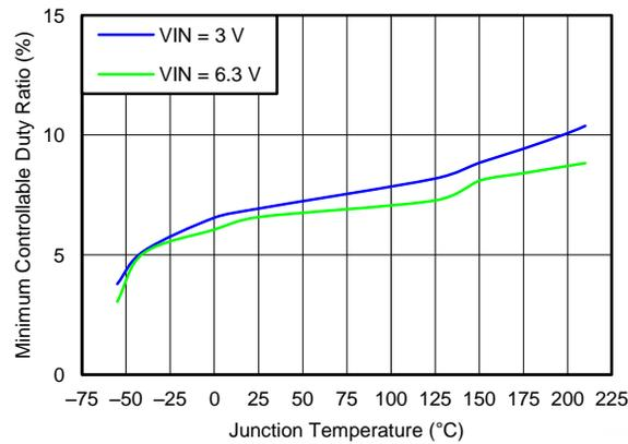
**Figure 16. Minimum Controllable Duty Ratio vs Temperature**
