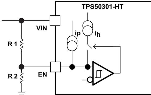
Figure 18. Adjustable VIN UVLO
