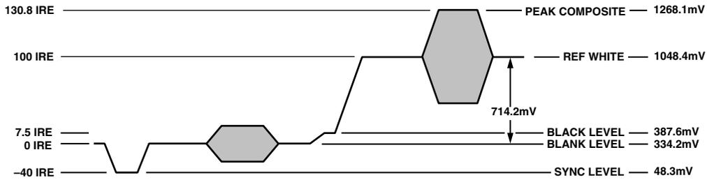
Figure 49. NTSC Composite Video Levels
