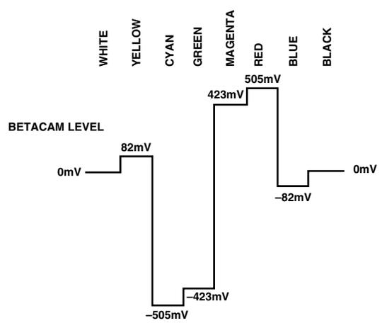
Figure 64. NTSC 100% Color Bars No Pedestal V Levels
