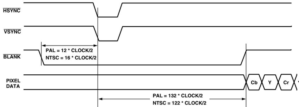
Figure 23. Timing Mode 2 Even-to-Odd Field Transition Master/Slave
