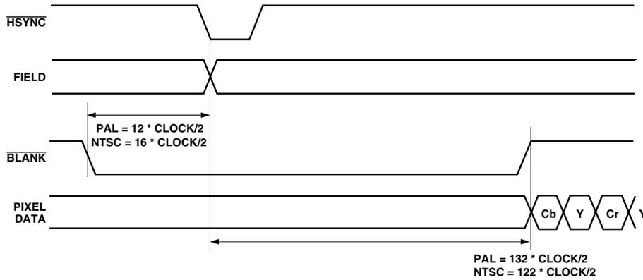
Figure 20. Timing Mode 1 Odd/Even Field Transitions Master/Slave
