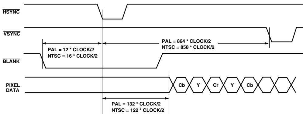
Figure 24. Timing Mode 2 Odd-to-Even Field Transition Master/Slave
