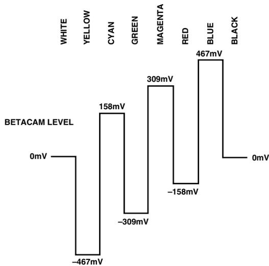
Figure 62. NTSC 100% Color Bars with Pedestal U Levels
