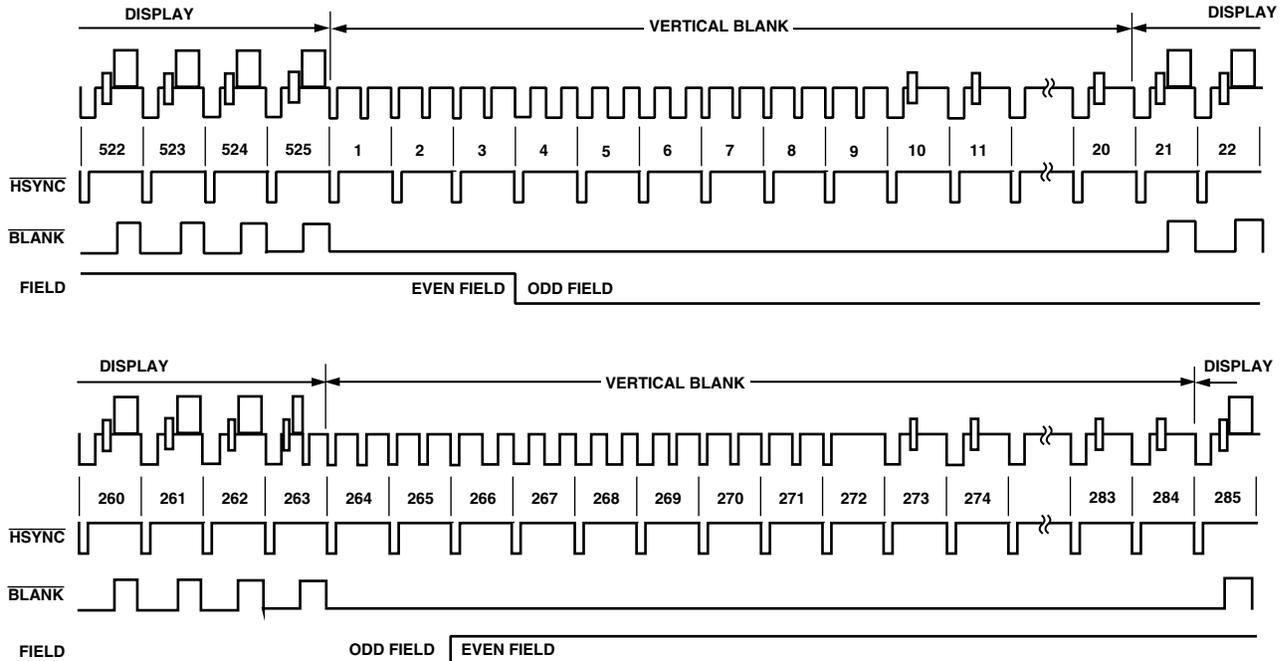
Figure 18. Timing Mode 1 (NTSC)
