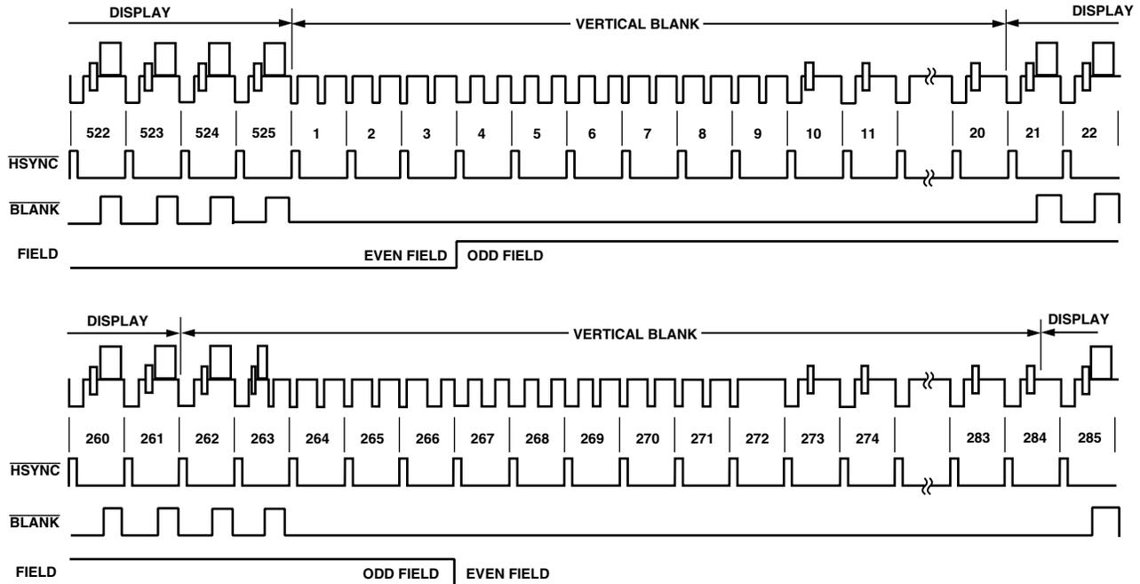
Figure 25. Timing Mode 3 (NTSC)
