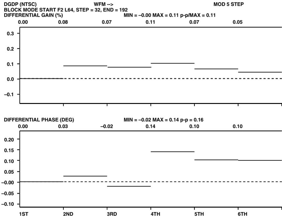
Figure 80. NTSC Differential Gain and Phase Measurement
