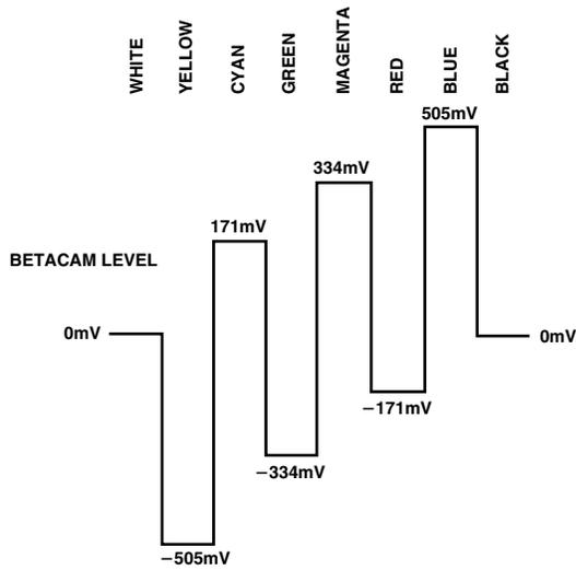
Figure 61. NTSC 100% Color Bars No Pedestal U Levels
