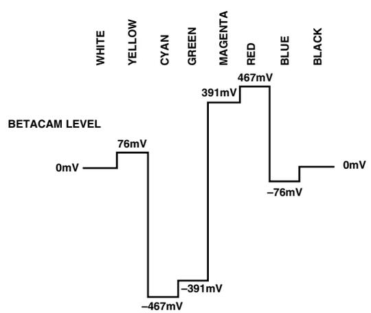
Figure 65. NTSC 100% Color Bars with Pedestal V Levels
