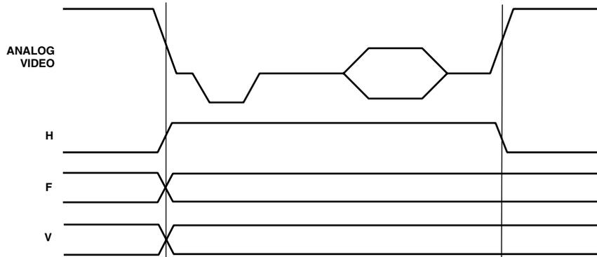
Figure 17. Timing Mode 0 Data Transitions (Master Mode)
