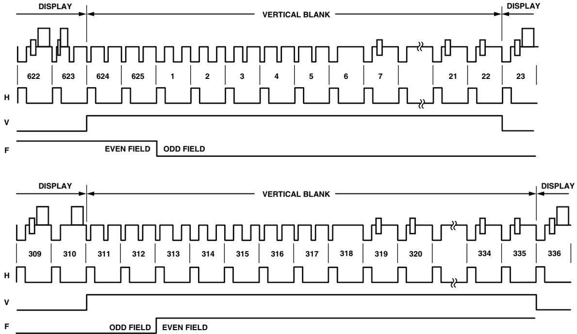
Figure 16. Timing Mode 0 (PAL Master Mode)
