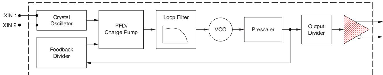
Figure 1. CDC421Axxx: High-Level Block Diagram
