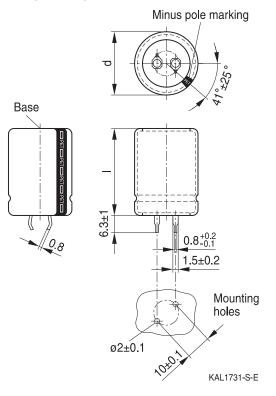
Snap-in terminals, length (6.3  $\pm 1$ ) mm. Also available in a shorter version with a length of (4.5 -1) mm.
