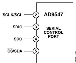
Figure 52. Serial Control Port
