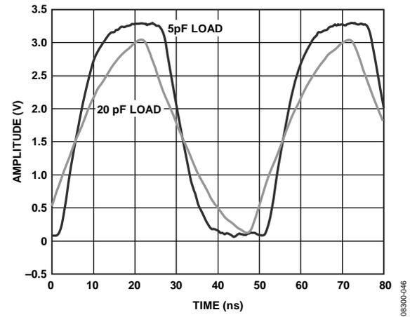
Figure 24. Output Waveform, 3.3 V CMOS (20 MHz, Weak Mode)
