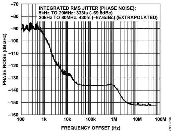
Figure 4. Absolute Phase Noise (Output Driver = LVPECL),
