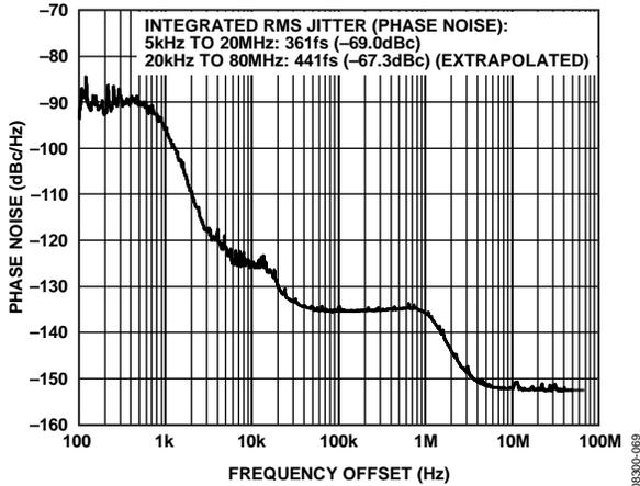
Figure 7. Absolute Phase Noise (Output Driver = LVPECL),
