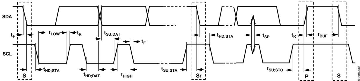
Figure 65. I<sup>2</sup>C Serial Port Timing
