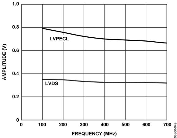
Figure 13. Amplitude vs. Toggle Rate, LVPECL and LVDS
