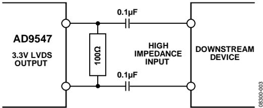
Figure 26. AC-Coupled LVDS or LVPECL Output Driver
