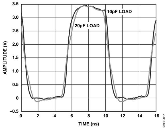
Figure 21. Output Waveform, 3.3 V CMOS (100 MHz, Strong Mode)
