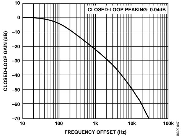
Figure 12. Jitter Transfer Bandwidth, Output Driver = LVPECL,
