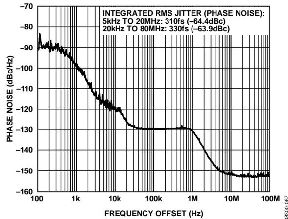
Figure 6. Absolute Phase Noise (Output Driver = LVPECL),
