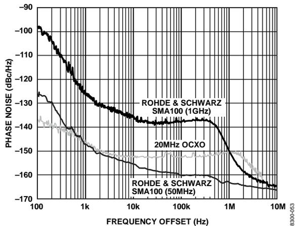
Figure 9. Phase Noise of SYSCLK Input Sources
