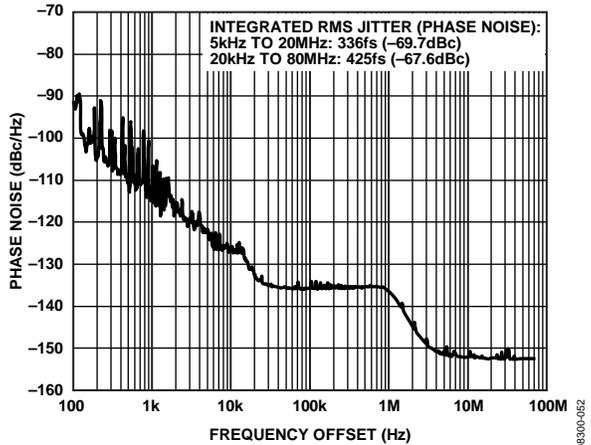
Figure 11. Absolute Phase Noise (Output Driver = LVPECL),
