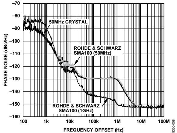
Figure 10. Absolute Phase Noise Comparison of SYSCLK Input Options
