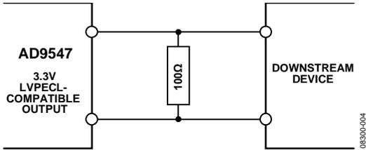
Figure 27. DC-Coupled LVDS or LVPECL Output Driver
