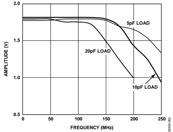
Figure 16. Amplitude vs. Toggle Rate, 1.8 V CMOS
