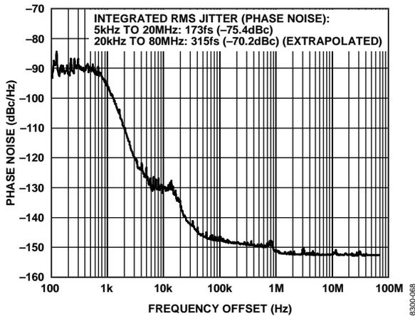
Figure 3. Absolute Phase Noise (Output Driver = LVPECL),
