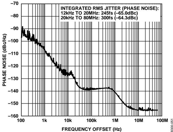
Figure 8. Absolute Phase Noise (Output Driver = LVPECL),
