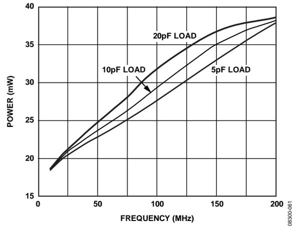
Figure 18. Power Consumption vs. Frequency, 1.8 V CMOS
