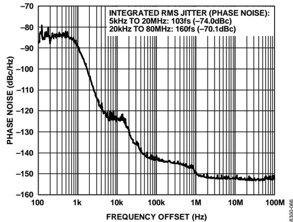
Figure 5. Absolute Phase Noise (Output Driver = LVPECL),
