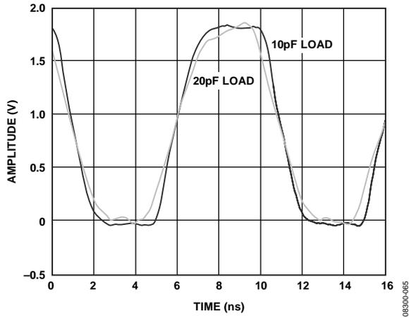
Figure 25. Output Waveform,
