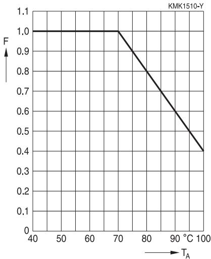
Maximum  $I_{\text{RMS}}$  current as function of the ambient temperature:  $I_{\text{RMS}}(T_A) = \text{Factor} \times I_{\text{RMS}}(70\text{ °C})$
