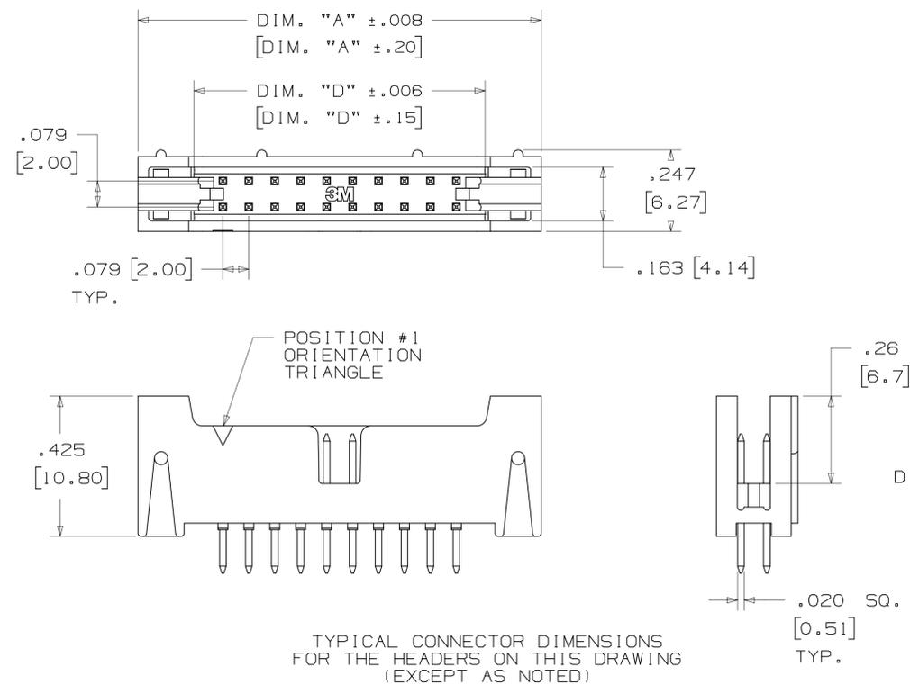
TYPICAL CONNECTOR DIMENSIONS FOR THE HEADERS ON THIS DRAWING (EXCEPT AS NOTED)
