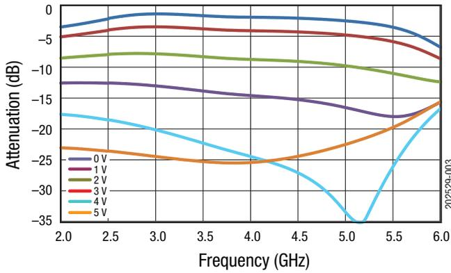
Figure 3. Attenuation vs Frequency Over Control Voltage
