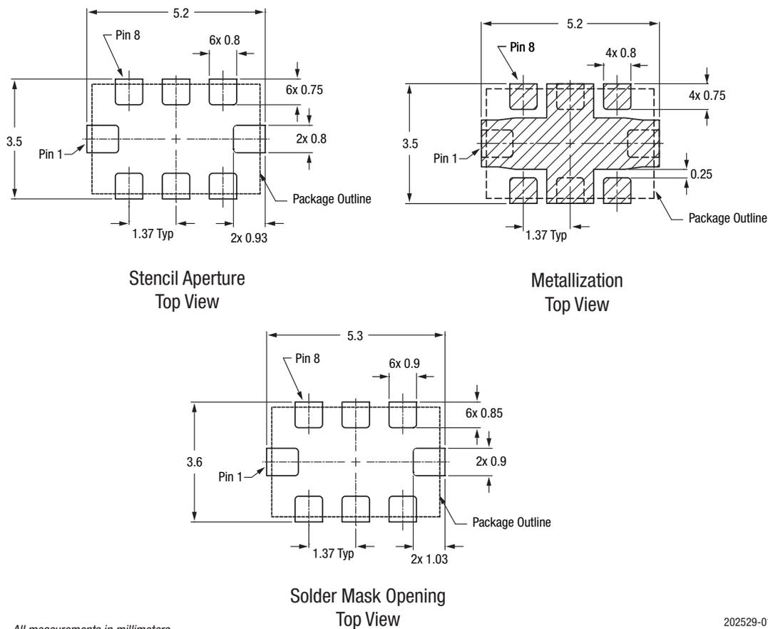
All measurements in millimeters
