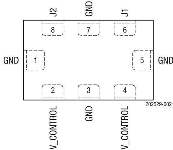
**Figure 2. SKY12236-11 Pinout (Top View)**
