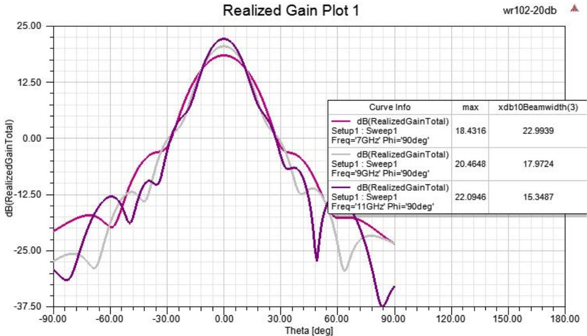
WR-102 Standard Gain Horn with 20 dBi gain, End Launch N Female connector from Pasternack Enterprises has same day shipment for domestic and International orders. Our RF, microwave and millimeter wave products maintain a 99.4% availability and are part of the broadest selection in the industry.
