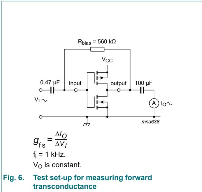
**Fig. 6. Test set-up for measuring forward transconductance**
