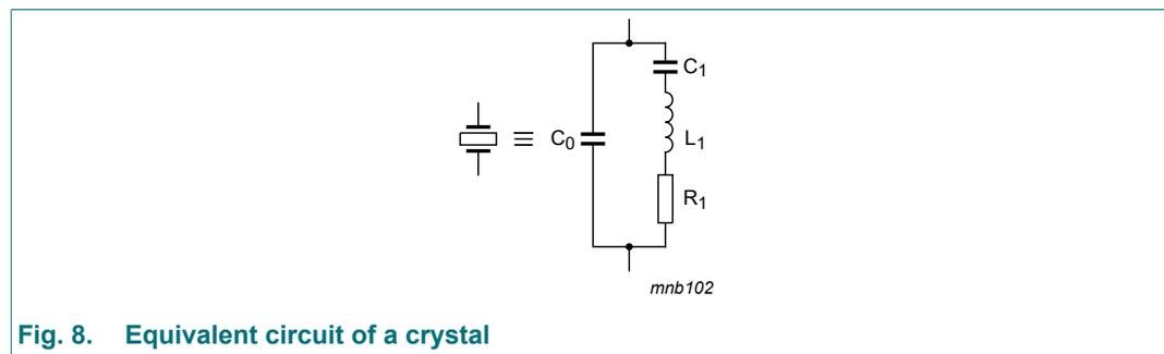
**Fig. 8. Equivalent circuit of a crystal**
