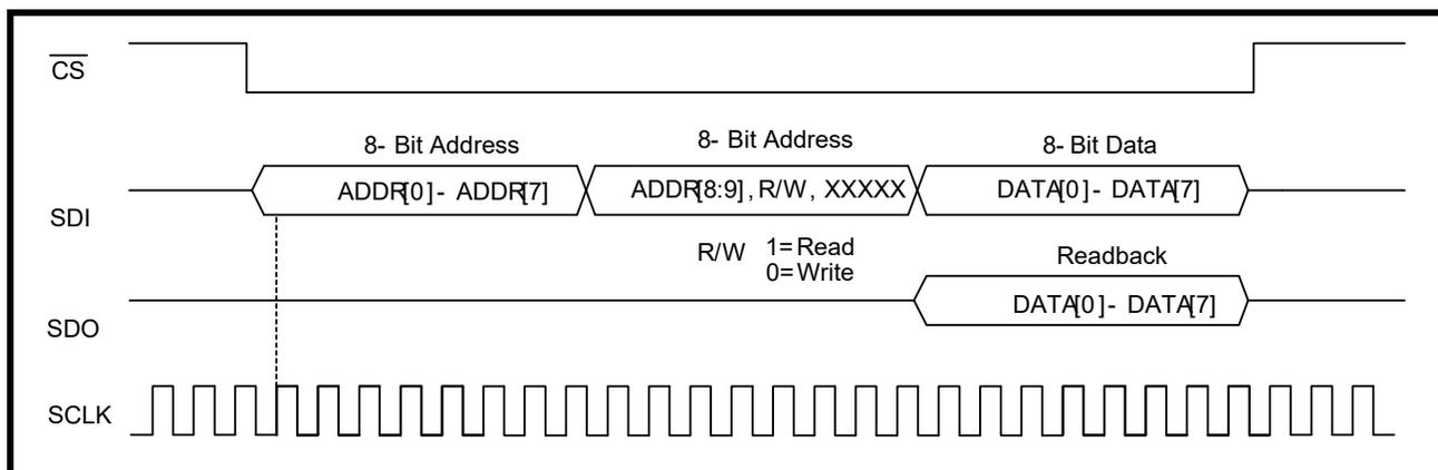
**NOTE:** For applications without a free running SCLK, a minimum of 1 SCLK pulse must be applied when  $\overline{\text{CS}}$  is "High", before pulling  $\overline{\text{CS}}$  "Low".
