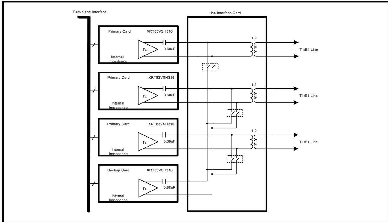
**5.3.6 Receive Interface with N+1 Redundancy**
