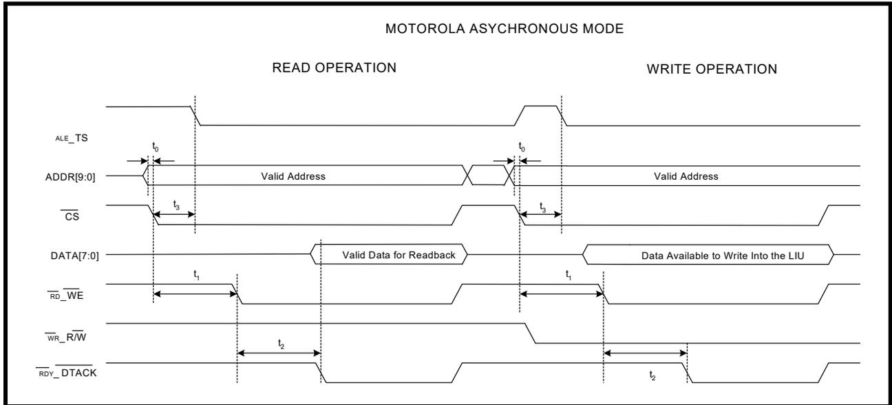
**TABLE 22: MOTOROLA 68K MICROPROCESSOR INTERFACE TIMING SPECIFICATIONS**
