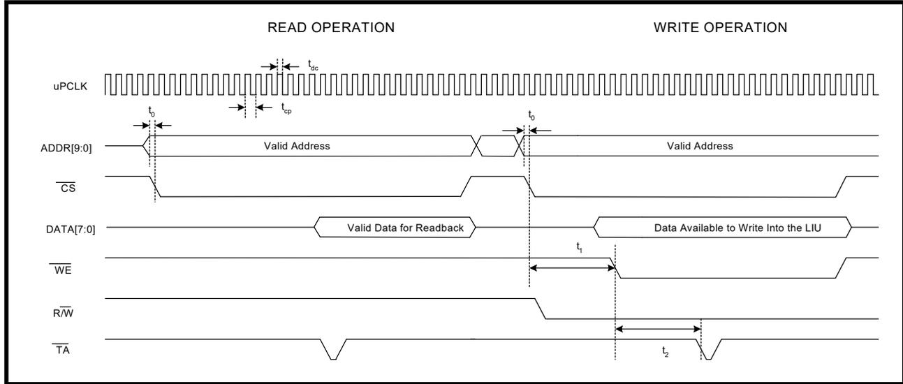
TABLE 21: MOTOROLA MPC86X MICROPROCESSOR INTERFACE TIMING SPECIFICATIONS
