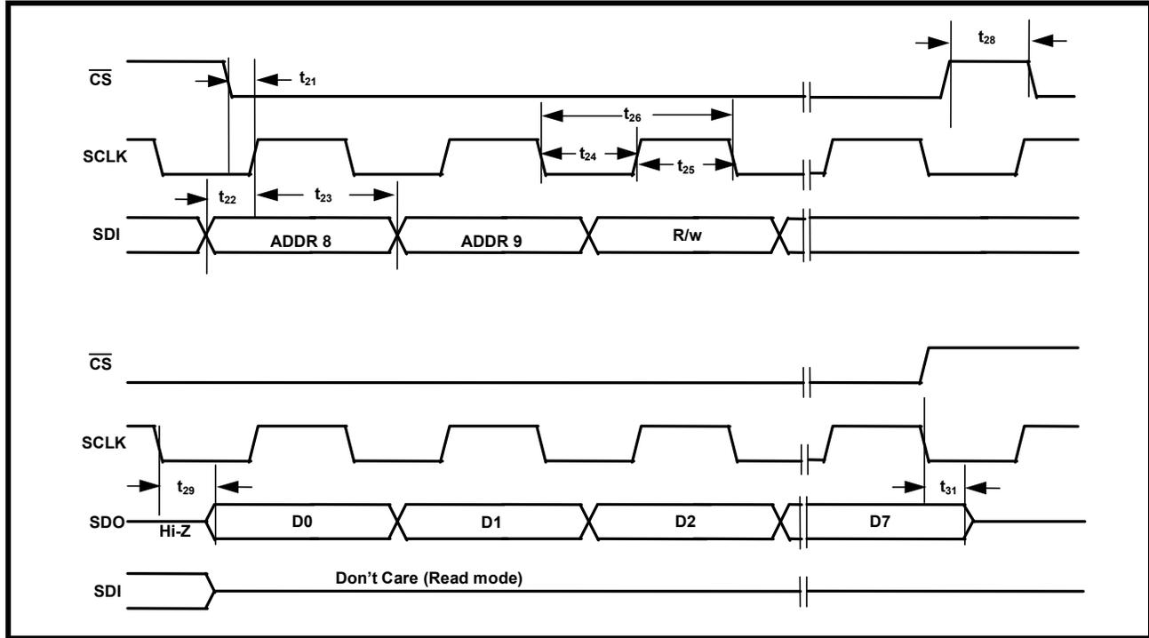
TABLE 14: MICROPROCESSOR SERIAL INTERFACE TIMINGS (  $T_A = 25^{\circ}C$ ,  $V_{DD} = 3.3V \pm 5\%$  AND LOAD = 10PF)
