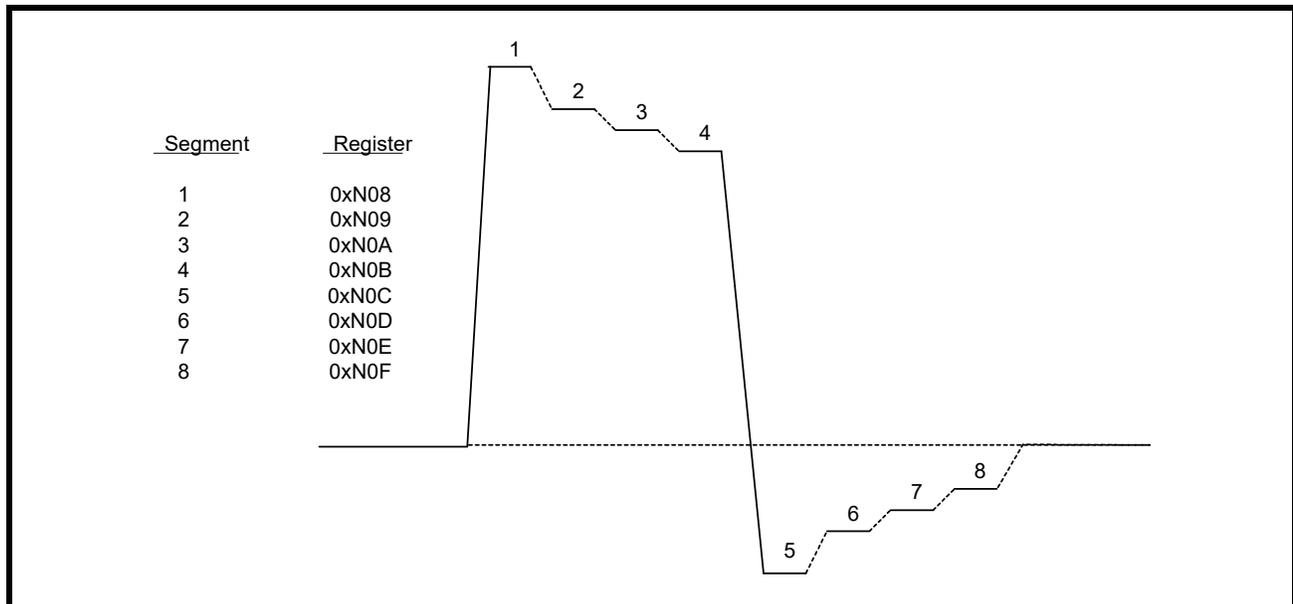
**NOTE:** By default, the arbitrary segments are programmed to 0x00h. The transmitter outputs will result in an all zero pattern to the line interface.
