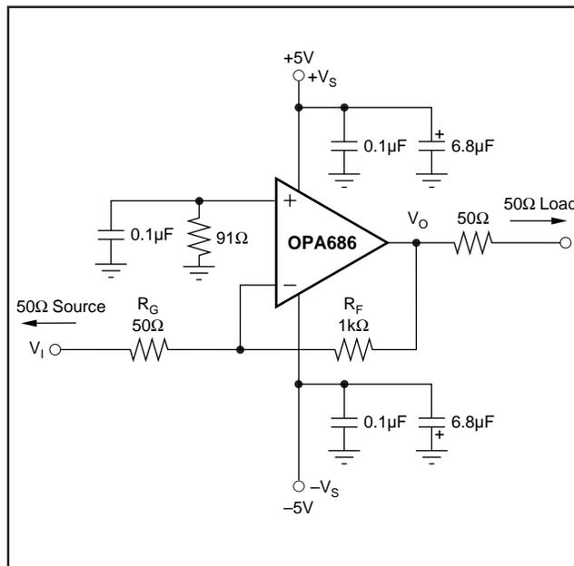
FIGURE 2. Inverting,  $G = -20$  Characterization Circuit.
