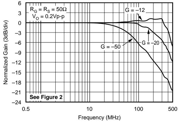
NON-INVERTING LARGE-SIGNAL FREQUENCY RESPONSE
