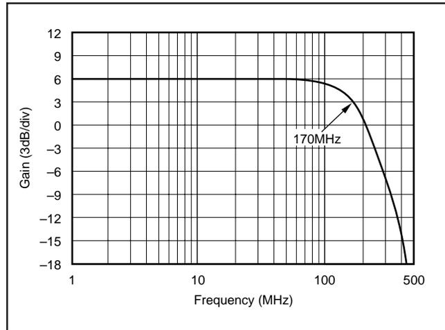
FIGURE 5.  $G = -2$  Frequency Response with External Compensation.
