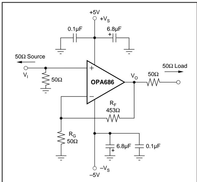
FIGURE 1. Non-Inverting,  $G = +10$  Specification and Test Circuit.
