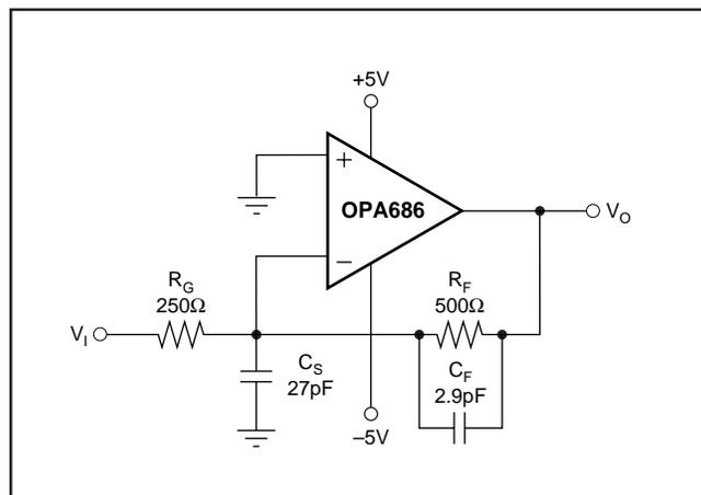
FIGURE 4. Broadband Low Gain Inverting External Compensation.
