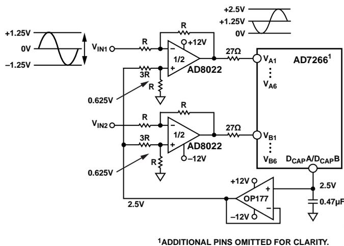
Figure 2. [AD8022](#) DC-Coupled Circuit for a Single-Ended Input Mode of Operation (Simplified Schematic; Decoupling and All Connections Not Shown)
