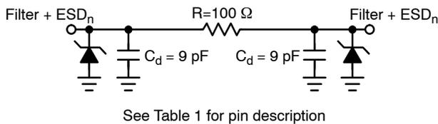
Figure 1. Electrical Schematic
